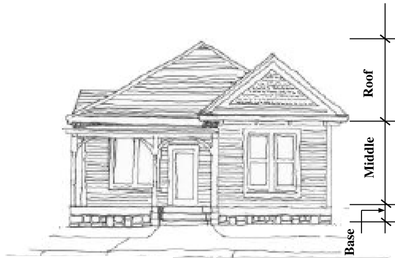
FIGURE 6-4 EXPRESSION OF BASE, MIDDLE AND ROOF ELEMENTS
