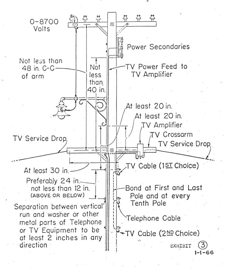
Telephone Pus Carrying Open Wire c Cable or Both
