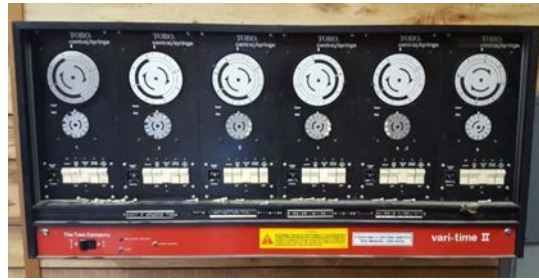
Current TORO Vari-Time II Central Controller
