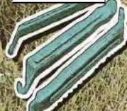
Tire levers help with tire removal. Use cautiously if used to re-seat a tire to avoid repuncturing the tube.
