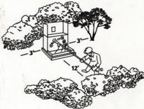
**We need room to work safely on this device. Please keep shrubs and structures 12 feet away from front side and 3 feet from other sides.**
