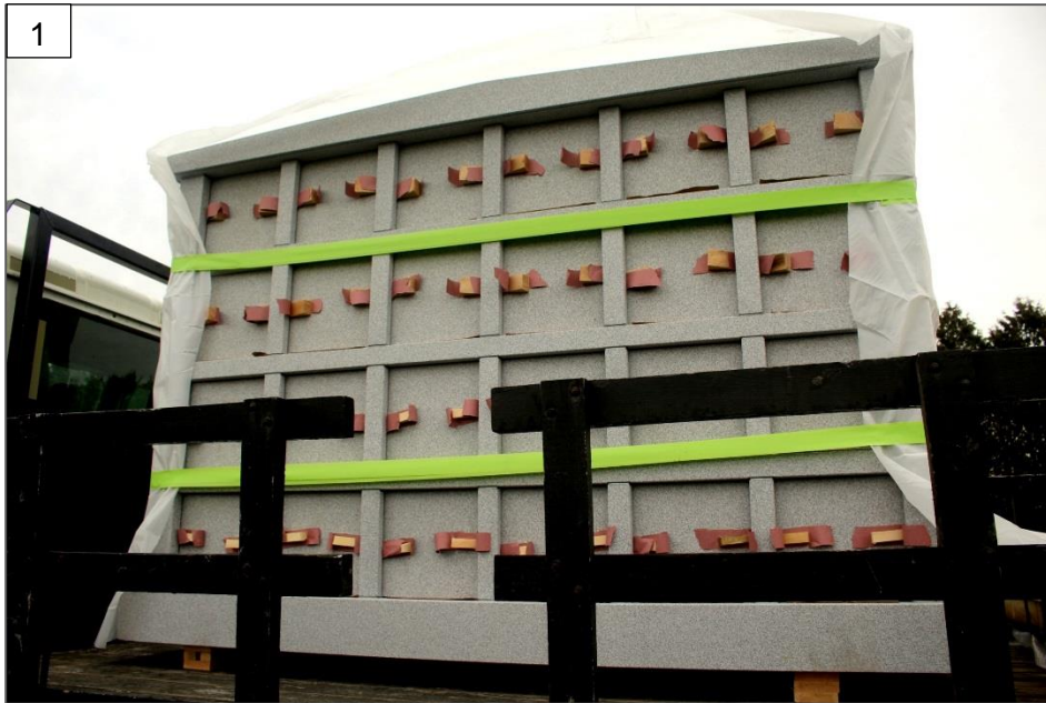
Photos taken 17 November 2023. Photo 1: Direct from the factory floor, the shutters have been braced with wood wedges and untreated building paper to keep them in place during transit over the rough roads. Photo 2: GCB Corp. did the work to set the columbarium. They spread out some hard rubber planking to help save the lawn from the heavy loads. Photo 3: a two-truck process, the one on the left brought the columbarium to the cemetery, the one on the right brought the heavy duty crane. Photo 4: With the two trucks in place, strap loops hanging from the hook on the end of the crane boom were slipped under the columbarium and it was lifted off of the truck. As seen in Photo 1, the columbarium traveled on blocks set on the bottom of the truck for easy strap placement.
