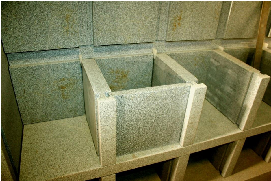
Above: status photo showing Columbarium 3 under construction. Mark Gherardi graciously invited Alan and I to the plant floor for a few photos of the construction progress. Photos taken 13 November. Below: a view of how a shutter fits onto the niche. The structure will be cleaned up prior to delivery.
