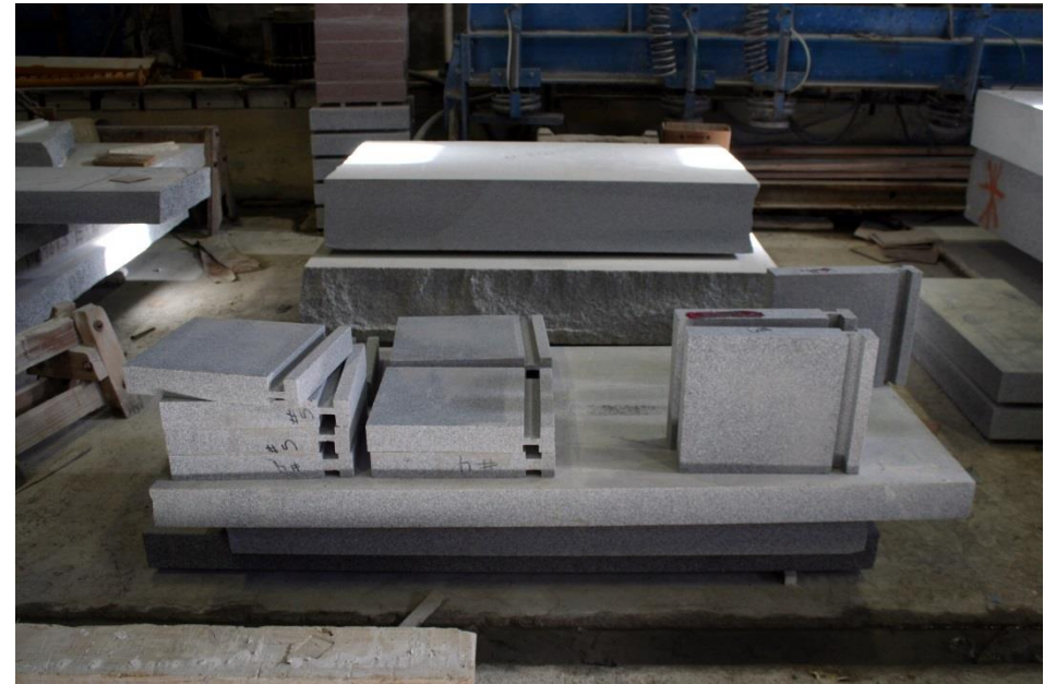
Above: The parts and pieces that make up the niches are held in place using some kind of epoxy and small plastic wedges while the epoxy dries. Below: an organized pile of parts and pieces awaiting assembly. Note the numbers on the individual pieces, these numbers correspond to those shown on the shop drawings provided to the cemetery commission.
