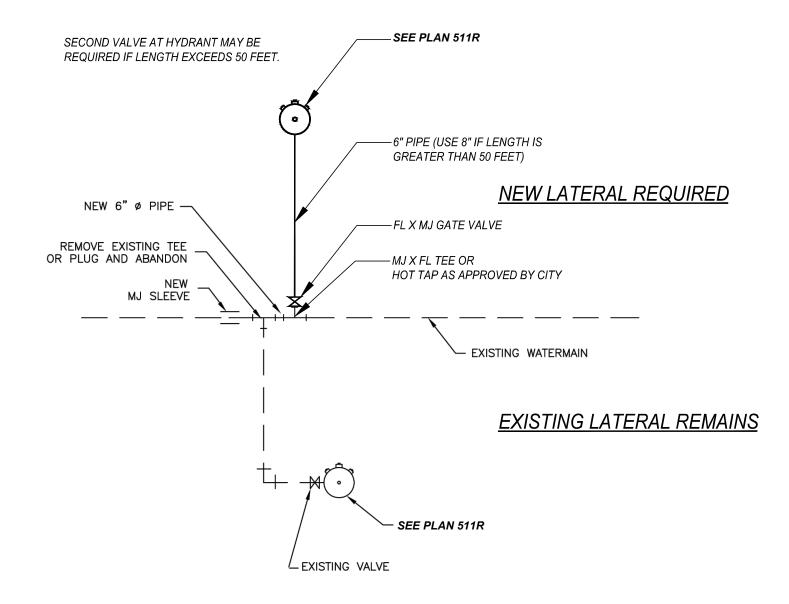
NOTE: THRUST BLOCKS REQUIRED (PLANS NO. 561R AND 562R)
