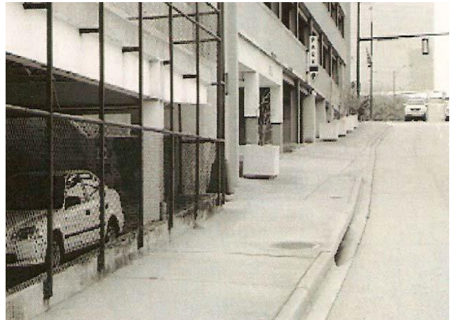
The visual impact of the cars themselves should be minimized. This parking structure does not provide any visual interest to passing pedestrians and is inappropriate.
