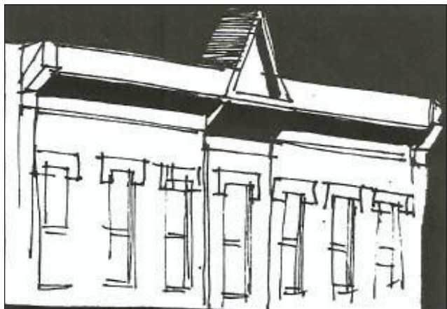
A simplified interpretation is also appropriate for a replacement cornice if evidence of the original is missing.
