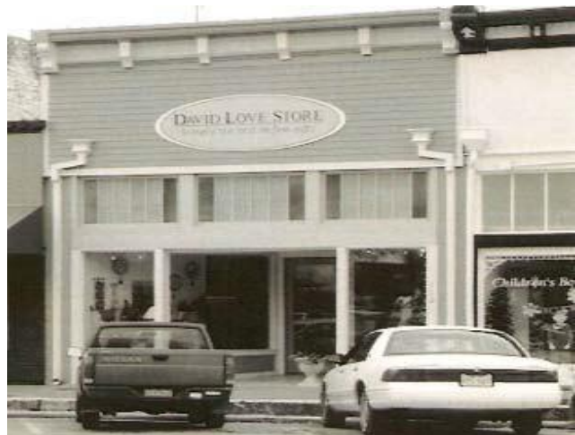
Locate a flush-mounted sign such that it fits within a panel formed by moldings or transom panels.
