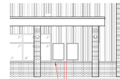
ELEVATION: WALK-UP WINDOW (UNLESS OTHERWISE DIRECTED) 2" INSET FROM MULLION 2" ABOVE STONE CAP 6" BETWEEN MENUS
