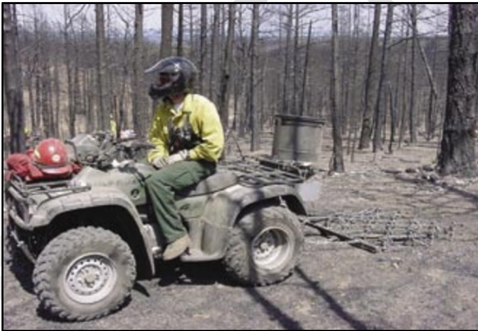
Figure G.15. ATV with scarifying tool attachment.
