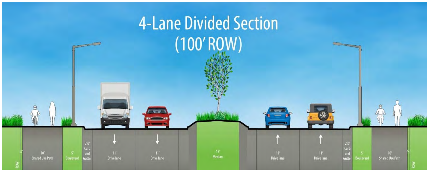
Figure 19: Urban 4-Lane Divided Typical Section
