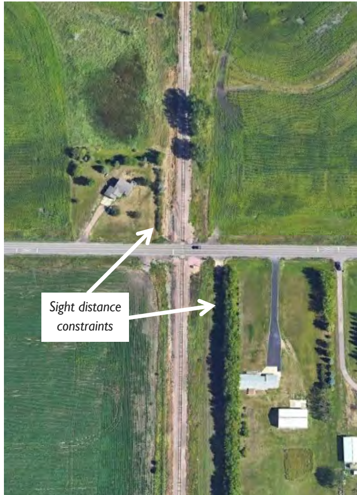
Figure 10: Railroad Crossing Sight Distance Constraints (Between Cliff Ave and Southeastern Ave)
