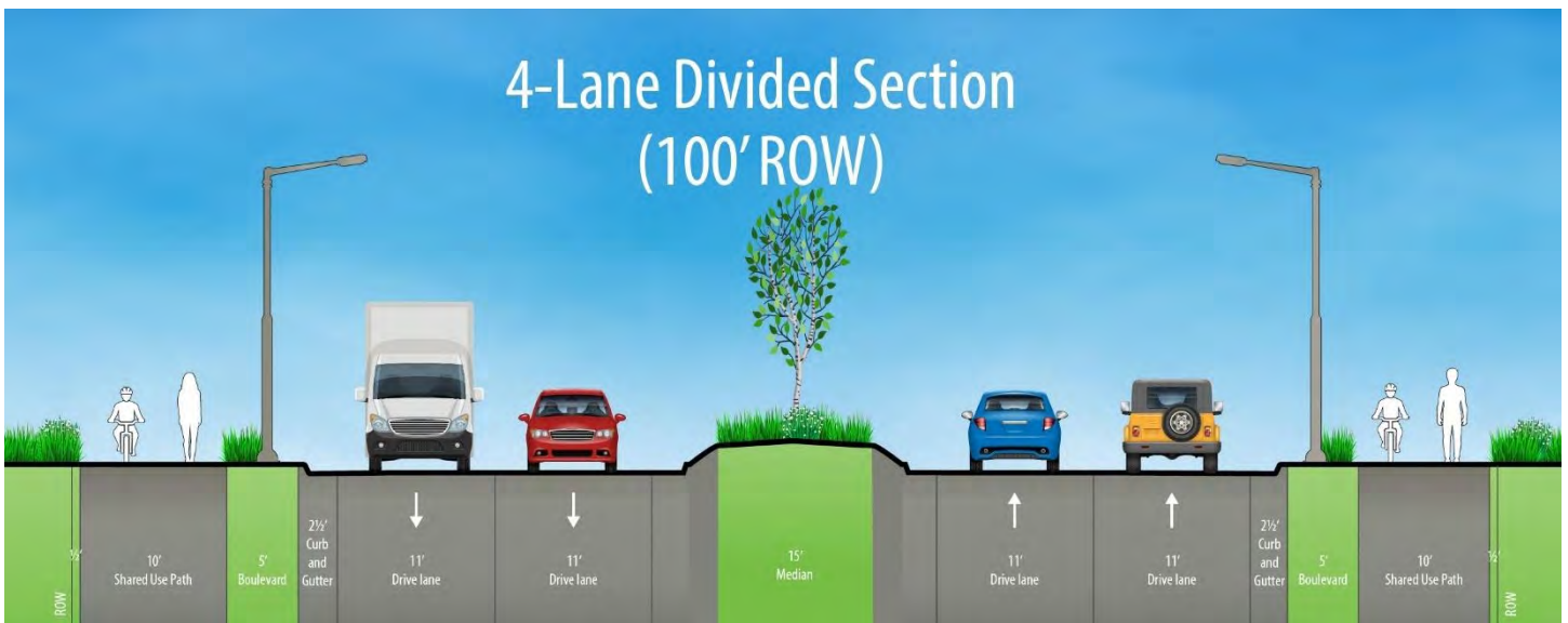
Figure 19: Urban 4-Lane Divided Typical Section
