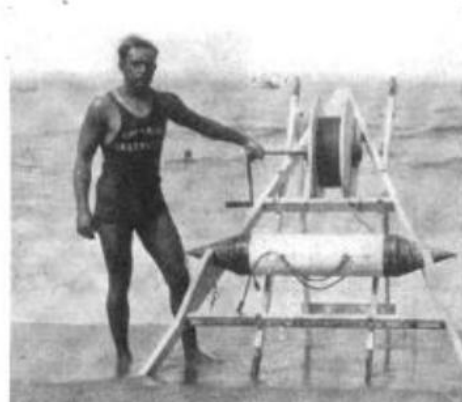
George Freeth with a life-saving buoy he designed, described as a “hollow, air-tight, copper torpedo forty-two inches by eight, which will hold up a dead weight of five-hundred pounds.”
