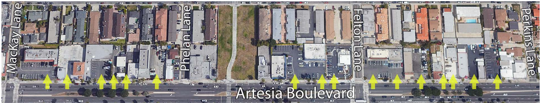
The three-block stretch (1,890 linear feet) of Artesia Boulevard between MacKay and Perkins Lanes has 16 curb cuts (see yellow arrows), an average of a curb cut every 120 feet. This is similar to curb-cut conditions throughout the Artesia Corridor.
