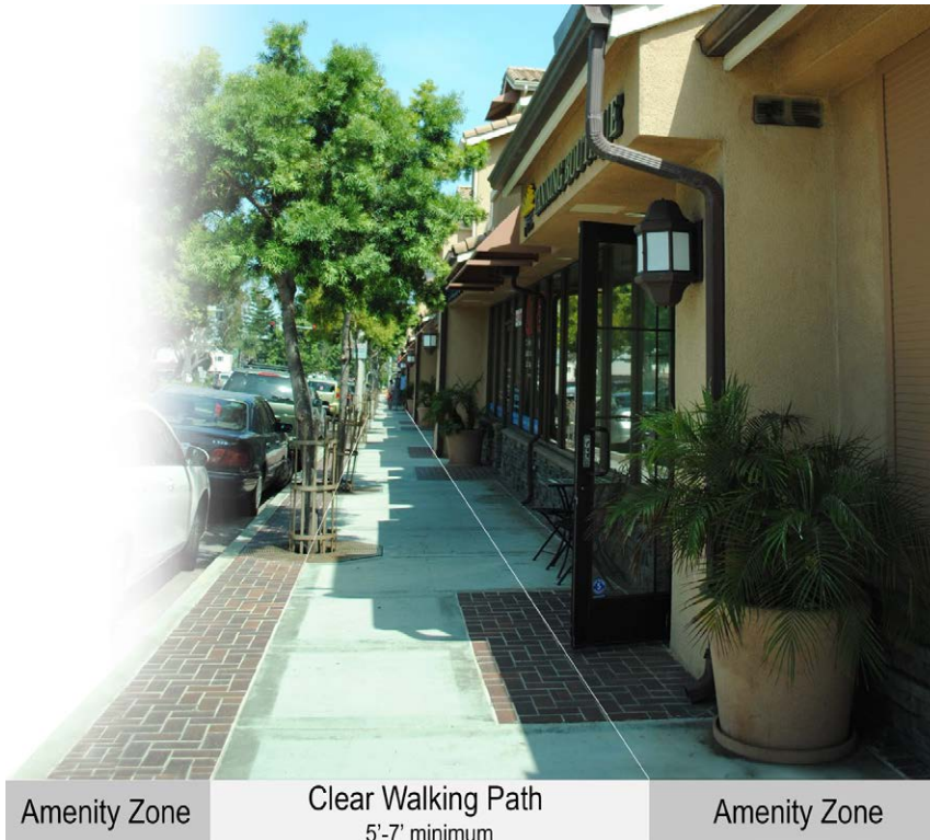
This sidewalk includes a clearly defined Clear Walking Path and two small Amenity Zones on either side. Here the Clear Walking Path is not linear, but rather curves around the street trees.
