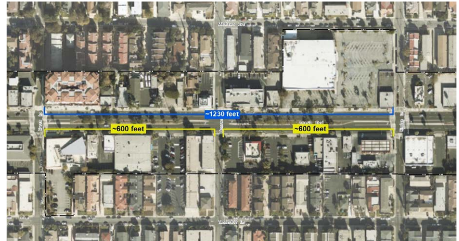
Example of average block lengths (600 feet) and maximum distance between crosswalks (1/4 mile).
