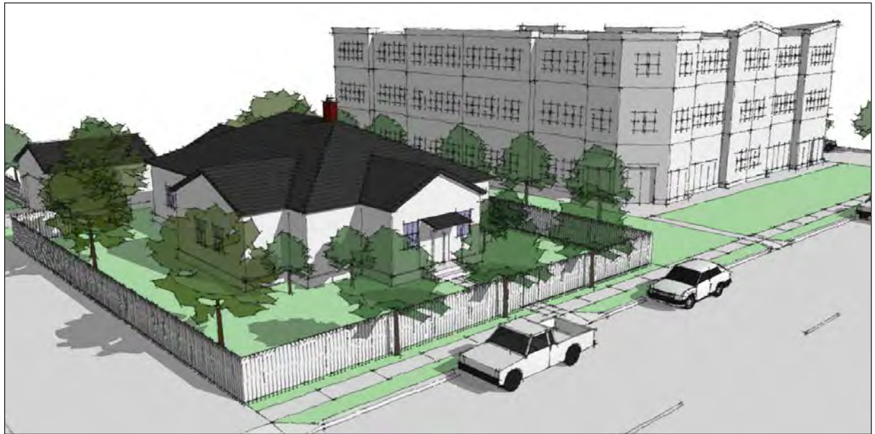
Even with conforming setbacks, building heights, and landscape buffers, the multiple family structure shown here is out of scale with the single family home.
