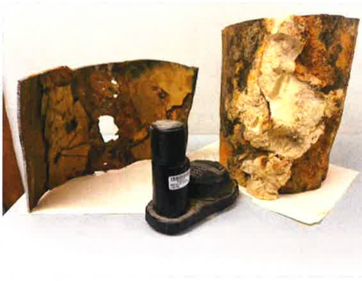
Figure 3: Perforation and corrosion on a segment of water main that was removed and replaced. This pipe had been installed in 1971 in the Downtown Loop.
