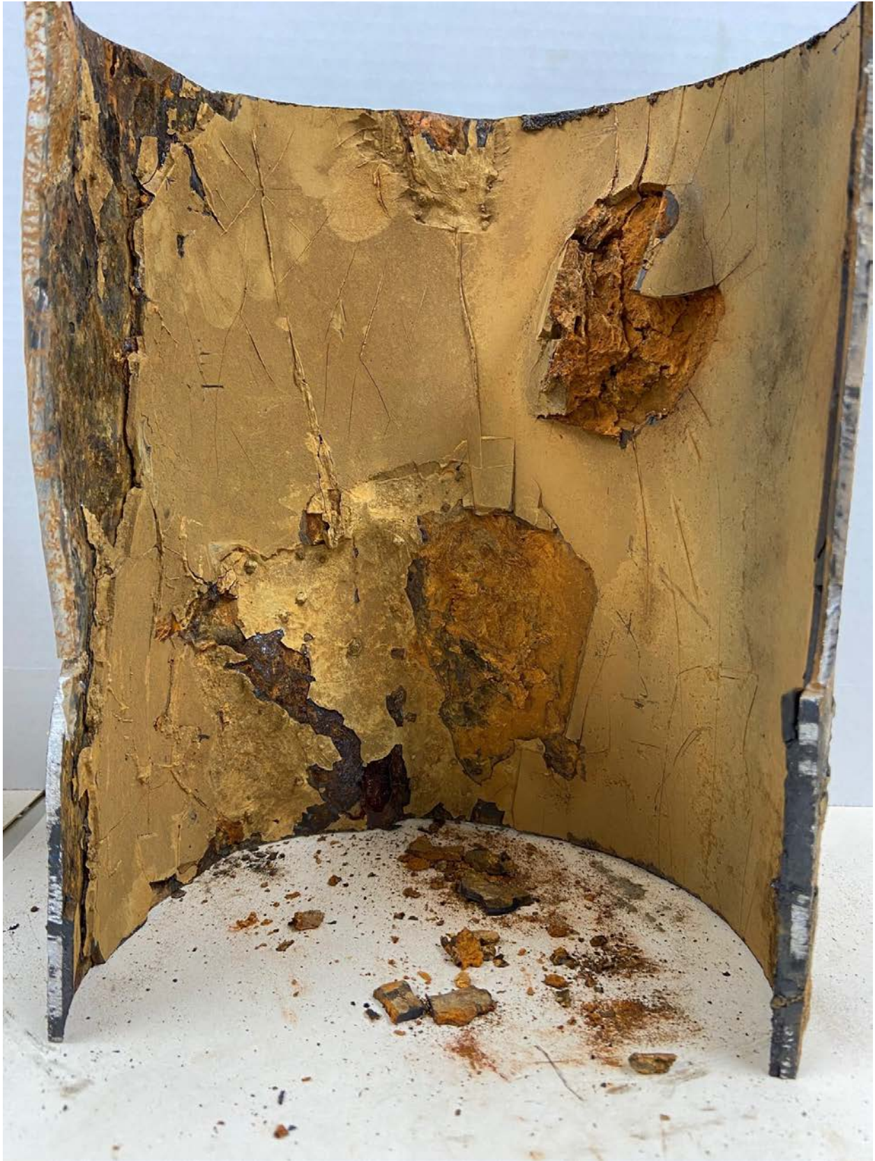
Sample of a steel water main salvaged by the Utility Department after the repair of a leak in the main.
