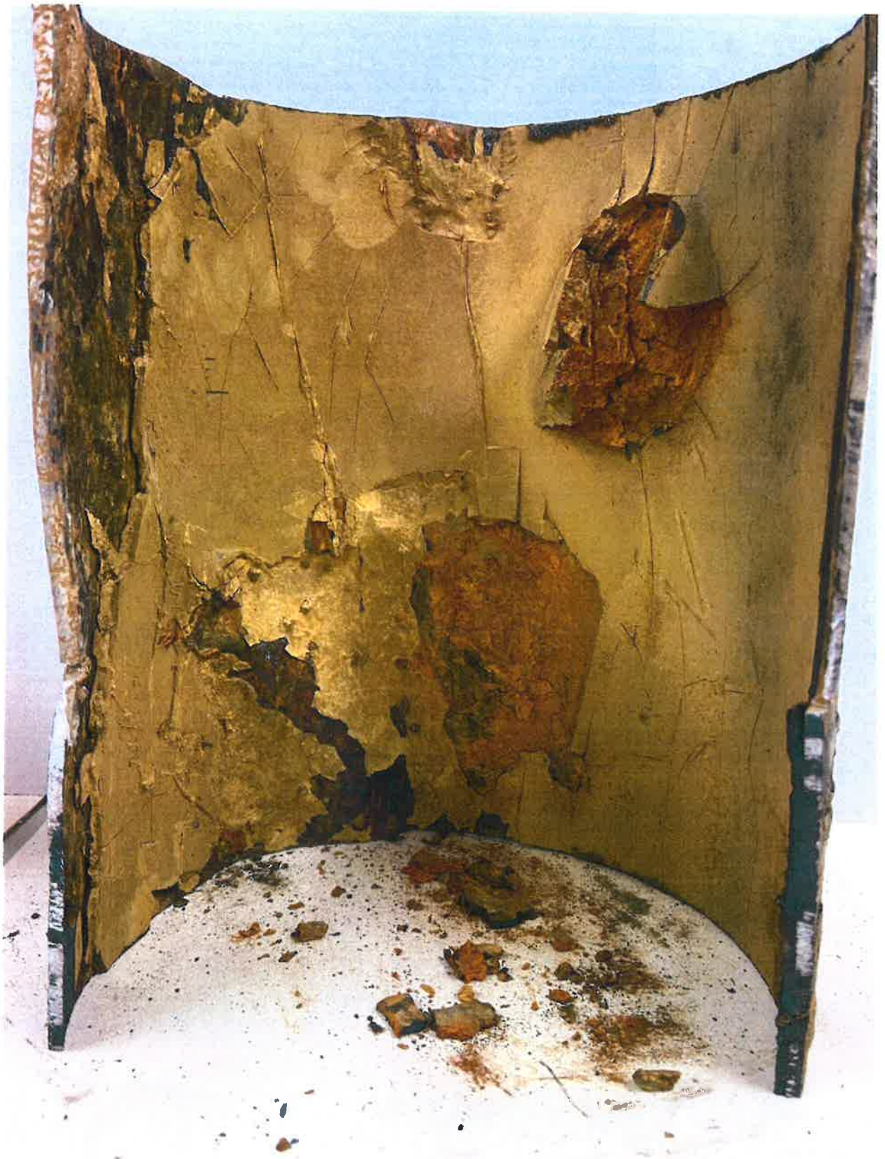
Sample of a steel water main salvaged by the Utility Department after the repair of a leak in the main.
