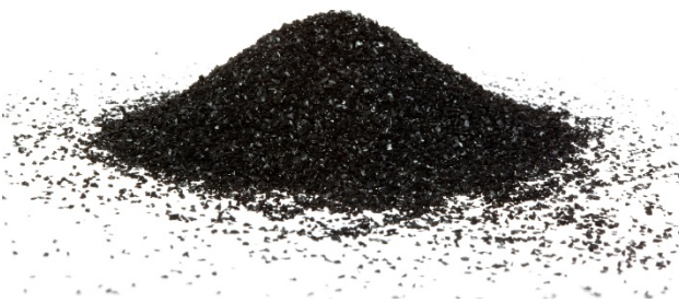
Example granular activated carbon media
