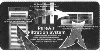
Wheeled Coach's air conditioning system retains the industry-leading benefits of our Pure Air Filtration System (P.A.F.) to protect your personnel from exposure to airborne particles 0.3 microns (Anthrax, Meningitis, TB) or larger at an efficiency rate of 99.97%.
