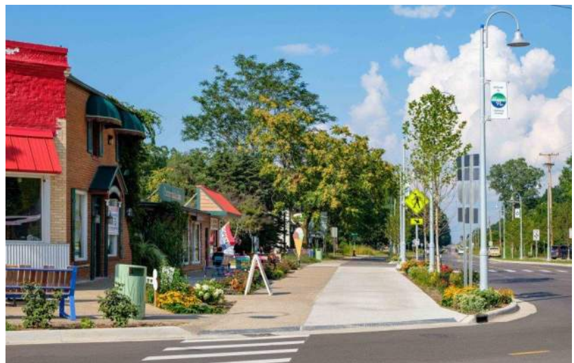
Figure 18: Shared Use Path with Adjacent Sidewalk
