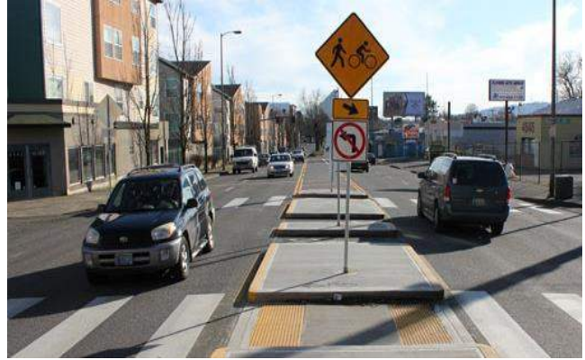
Figure 24: Pedestrian Refuge Island
