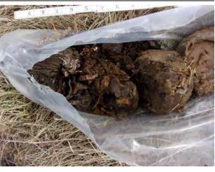
Clay cap (right) and top of refuse (left) from 1.5-2.5 feet bgs at SB-19 (4/12/2022).
