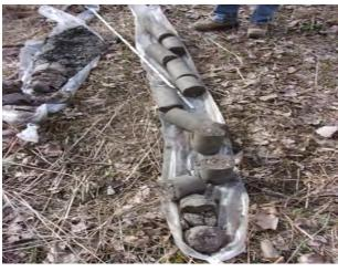
Very hard till clay from 10-15 feet bgs at MW-202 (4/12/2022).
