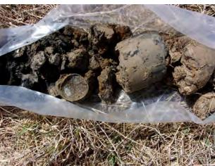
Clay cap (right) and top of refuse (left) at 1.5-3 feet bgs at SB-20 (4/12/2022).
