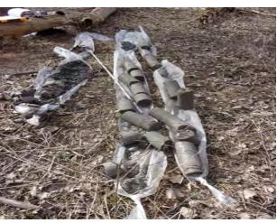
MW-202 soil cores from 0-30 feet bgs (4/12/2022). Zero feet bgs at top left. 30 feet bgs at lower right.
