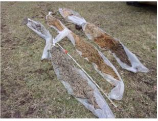
Soil cores from 0-30 feet bgs at MW-201 (4/11/2022). Zero feet bgs is at top right. 30 feet bgs is at bottom left.
