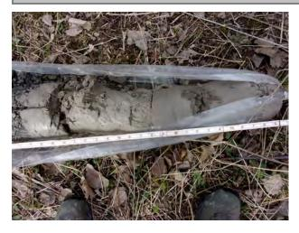
Very hard till clay from 8.5-10 feet bgs at MW-202 (4/12/2022).
