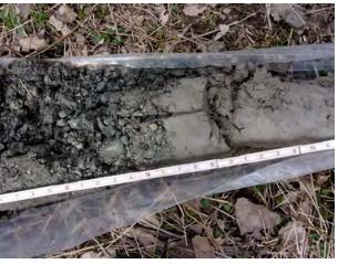
Contact of lacustrine sandy gravel (left) and clayey silt (right) at 7.7 feet bgs at MW-202 (4/12/2022).
