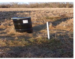
Containerized soil cores containing refuse from boring SB-20 (4/14/2022).
