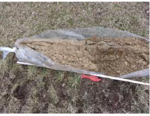
Contact of gravelly lacustrine sand (right) and fine grained lacustrine sand (left) at 8 feet bgs at MW-201 (4/11/2022).
