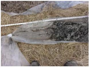
Lacustrine gravelly sand/very hard till clay contact at 33.5 feet bgs at SB-19 (4/12/2022).
