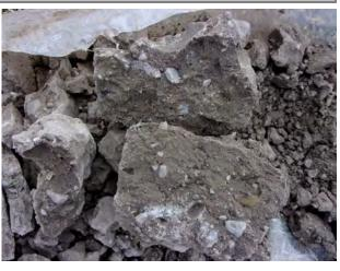
Hardpan-like till clay at 40 feet bgs at MW-201 (4/11/2022).
