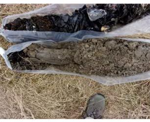
Fill sand and underlying refuse from 17-20 feet bgs at SB-19 (4/12/2022).
