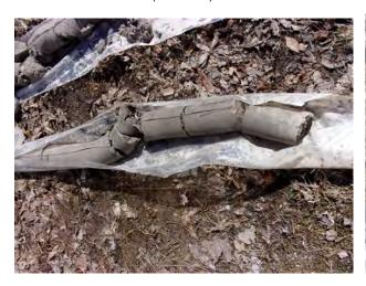
Till clay from 40-45 feet bgs at MW-200 (4/12/2022).
