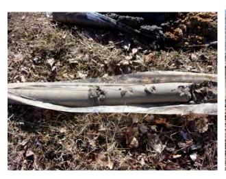
Till clay from 25.5-30 feet bgs at MW-200 (4/12/2022).
