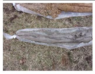
Till clay from 25-30 feet bgs at MW-201 (4/11/2022).
