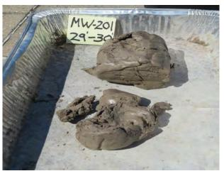
Till clay soil sample from 29-30 feet bgs at MW-201 (4/16/2022).
