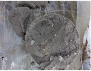
Hardpan-like till clay from 25-30 feet bgs at SB-21 (4/13/2022).
