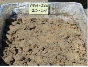
Lacustrine silty sand soil sample from 20-24 feet bgs at MW-201 (4/16/2022).
