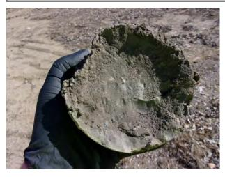
Hardpan-like till clay from 35-39.5 feet bgs at MW-200 (4/12/2022).
