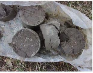
Till clay from 42-50 feet bgs at MW-201 (4/11/2022).
