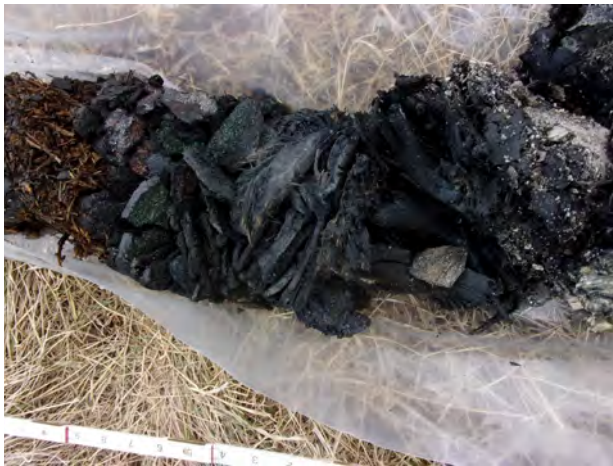
Refuse and wood from 5-10 feet bgs at SB-19 (4/12/2022).
