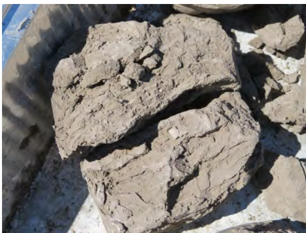
Till clay soil sample from 25.5-30 feet bgs at MW-200 (4/16/2022).
