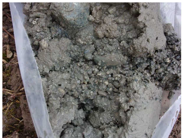
Lacustrine sandy gravel at 10 feet bgs at SB-21 (4/13/2022).
