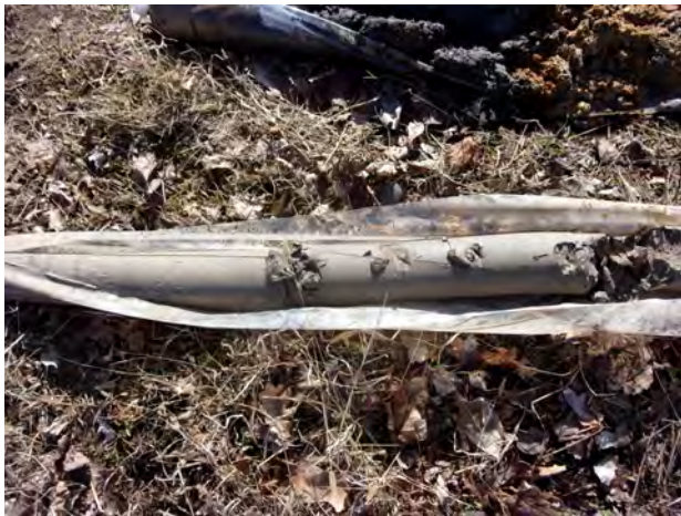
Till clay from 25.5-30 feet bgs at MW-200 (4/12/2022).
