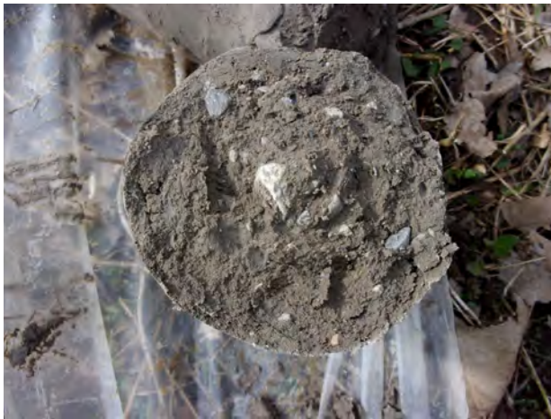
Very hard till clay at 10 feet bgs at MW-202 (4/12/2022).
