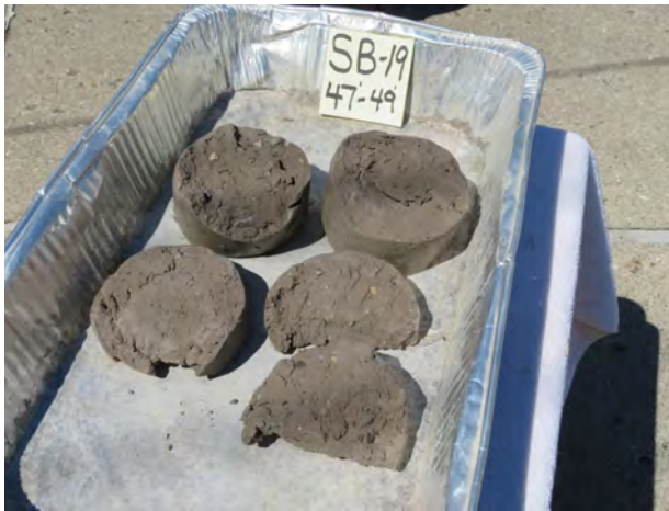
Till clay soil sample from 47-49 feet bgs at SB-19 (4/16/2022).
