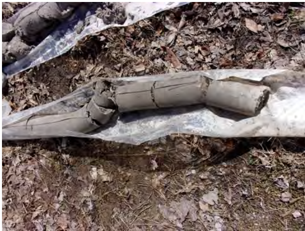
Till clay from 40-45 feet bgs at MW-200 (4/12/2022).
