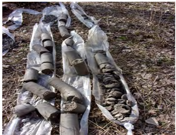
MW-202 soil cores from 20-40 feet bgs (4/12/2022). 20 feet bgs at top left. 40 feet bgs at lower right.
