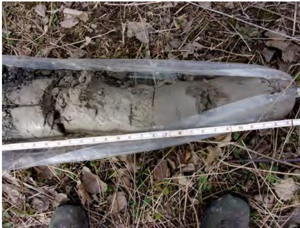
Very hard till clay from 8.5-10 feet bgs at MW-202 (4/12/2022).
