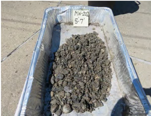
Lacustrine sandy gravel soil sample from 5-7 feet bgs at MW-202 (4/16/2022).
