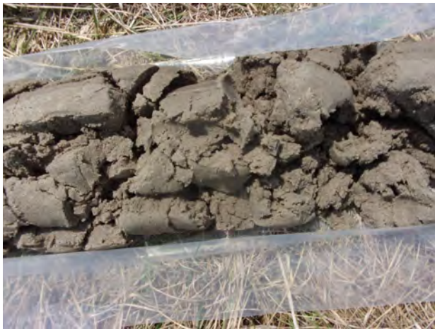
Lacustrine sand at 38 feet bgs at SB-20(4/12/2022).
