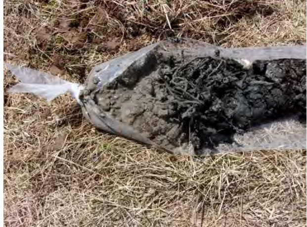
Base of refuse and top of lacustrine sand at 29-30 feet bgs at SB-20 (4/12/2022).
