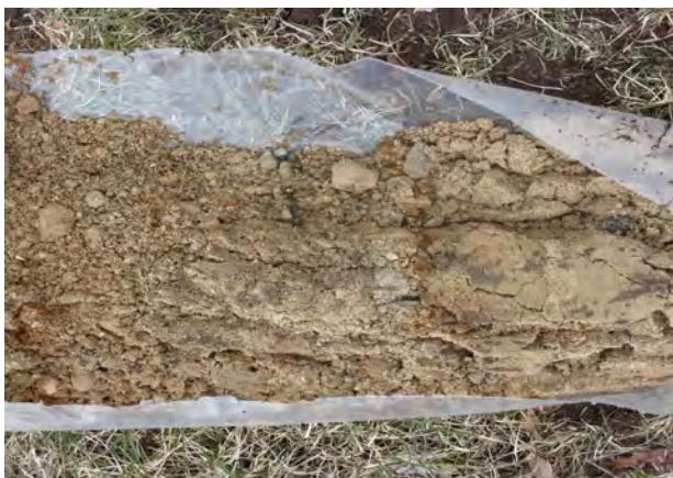
Contact of gravelly lacustrine sand (left) and fine grained lacustrine sand (right) at 8 feet bgs at MW-201 (4/11/2022).
