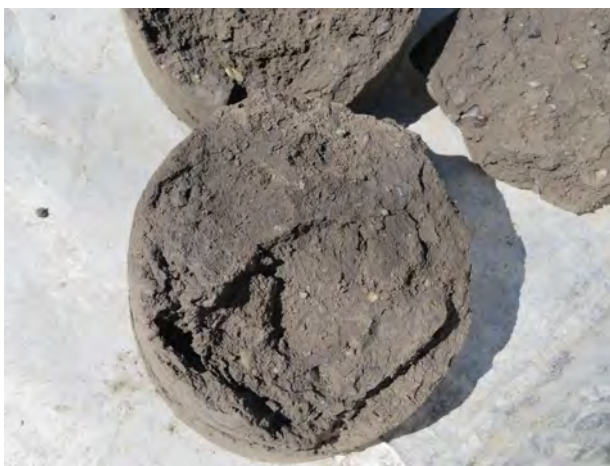
Till clay soil sample from 8.5-10 feet bgs at MW-202 (4/16/2022).
