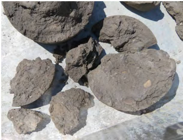
Till clay soil sample from 23-25 feet bgs at SB-21 (4/16/2022).
