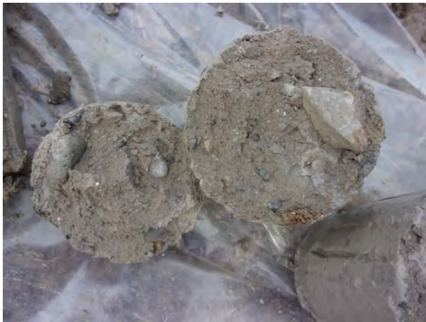
Very hard till clay from 15-20 feet bgs at SB-21 (4/13/2022).
