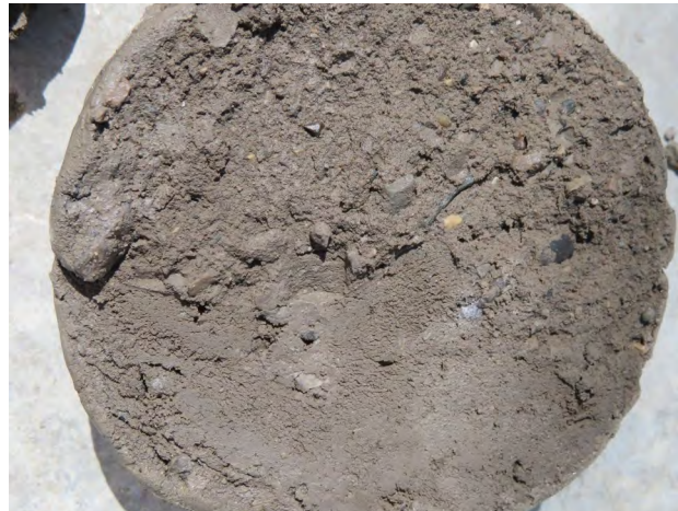
Very hard till soil sample (clayey sand) from 34-35 feet bgs at SB-19 (4/16/2022).
