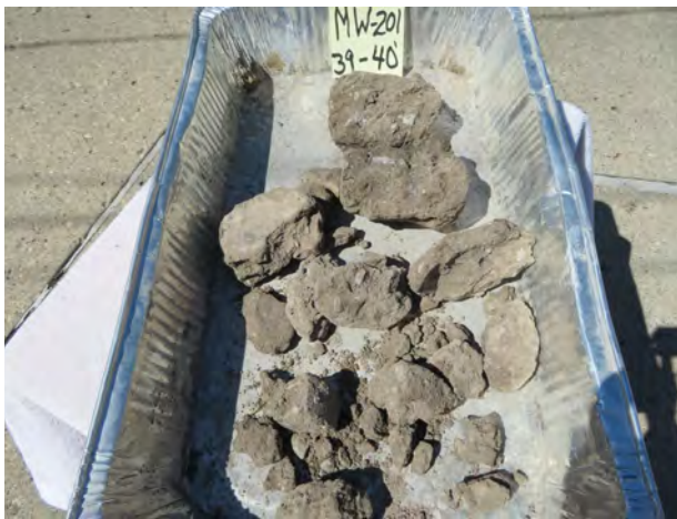
Hardpan-like till soil sample (silty-clayey sand) from 39-40 feet bgs at MW-201 (4/16/2022).
