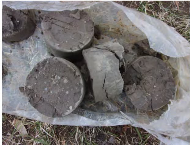
Till clay from 42-50 feet bgs at MW-201 (4/11/2022).
