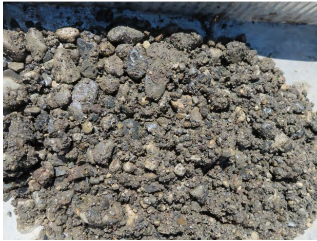
Lacustrine sandy gravel soil sample from 5-7 feet bgs at MW-202 (4/16/2022).
