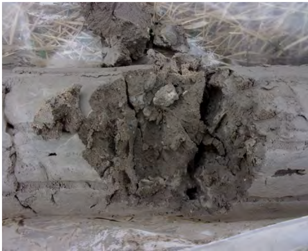
Very hard till clayey sand-sandy clay from 35-40 feet bgs at SB-19 (4/12/2022).
