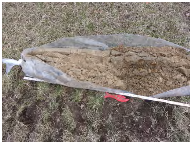
Contact of gravelly lacustrine sand (right) and fine grained lacustrine sand (left) at 8 feet bgs at MW-201 (4/11/2022).
