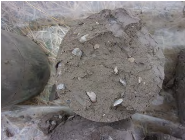
Very hard till clay from 40-50 feet bgs at SB-19 (4/12/2022).
