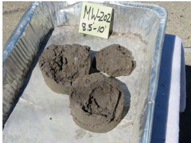
Till clay soil sample from 8.5-10 feet bgs at MW-202 (4/16/2022).
