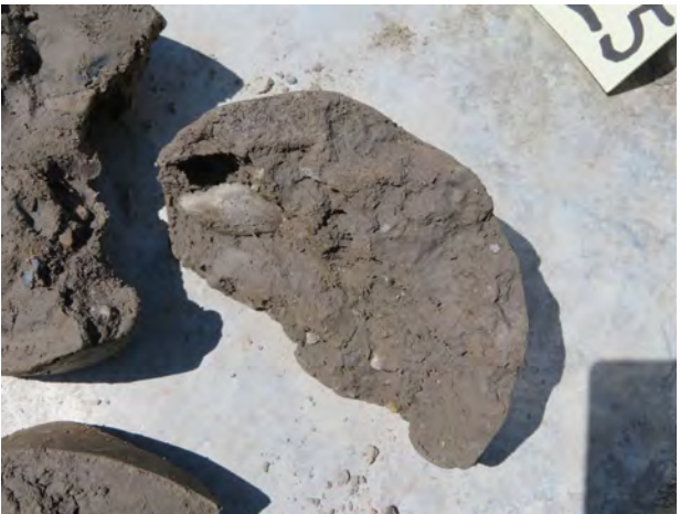
Till clay soil sample from 23-25 feet bgs at SB-21 (4/16/2022).
