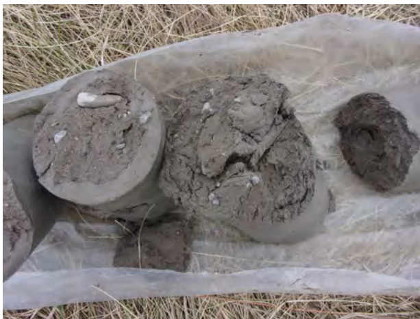
Very hard till clay from 40-50 feet bgs at SB-19 (4/12/2022).
