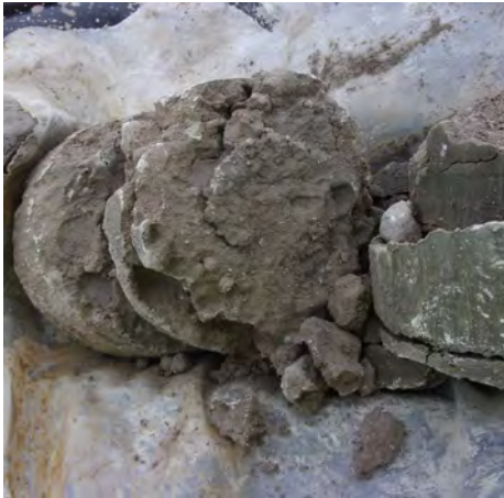
Hardpan-like glacial till from 76.5-80 feet bgs at MW-300 (4/4/2023).
