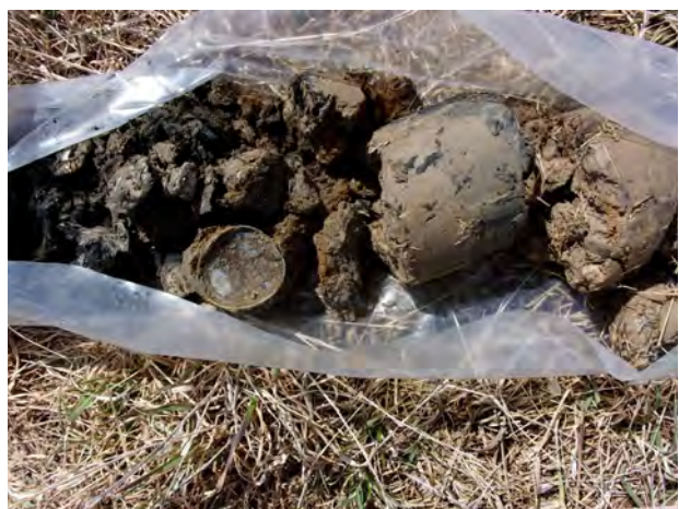
Clay cap (right) and top of refuse (left) at 1.5-3 feet bgs at SB-20 (4/12/2022).
