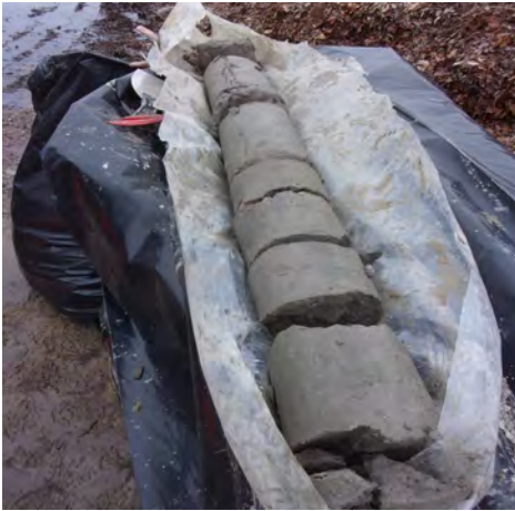
Very hard glacial till clay from 55-60 feet bgs at MW-300 (4/4/2023).
