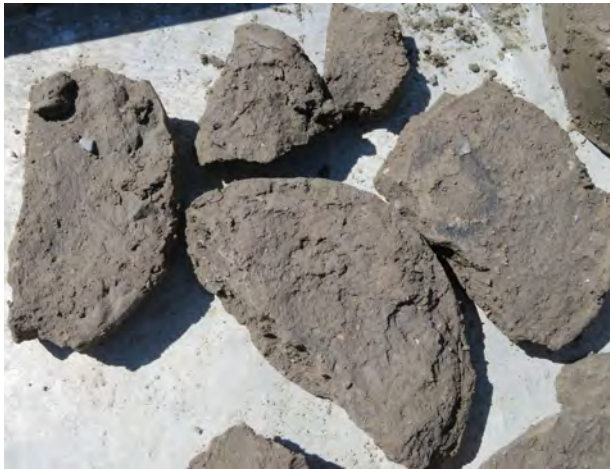
Till clay soil sample from 37-39.5 feet bgs at MW-200 (4/16/2022).
