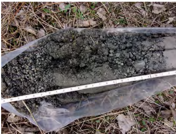
Lacustrine sandy gravel from 5-7.7 feet bgs at MW-202 (4/12/2022).
