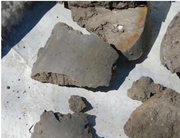
Till clay soil sample from 45-50 feet bgs at SB-20 (4/16/2022).
