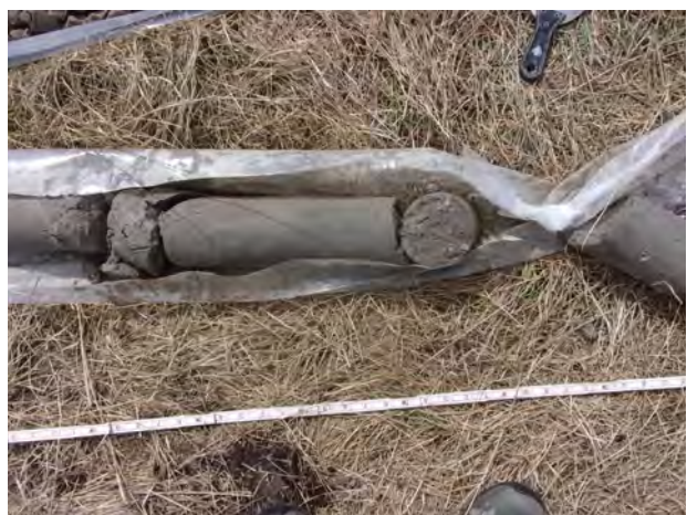
Hardpan-like till clay from 45-50 feet bgs at SB-20 (4/12/2022).
