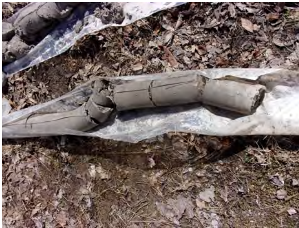
Till clay from 40-45 feet bgs at MW-200 (4/12/2022).
