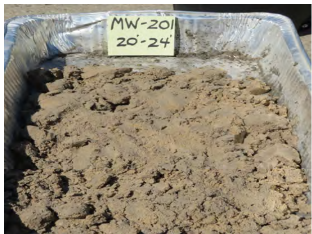
Lacustrine silty sand soil sample from 20-24 feet bgs at MW-201 (4/16/2022).
