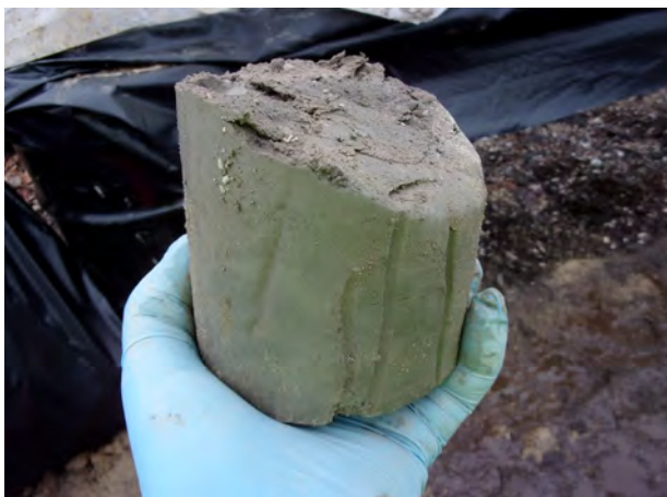
Hard glacial till clay from 30-35 feet bgs at MW-300 (4/4/2023).
