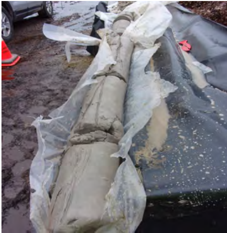
Hard glacial till clay from 25-30 feet bgs at MW-300 (4/4/2023).
