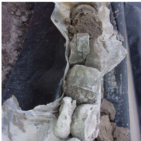
Hardpan-like glacial till from 79-81 feet bgs (just above boulder) at MW-300 (4/4/2023).
