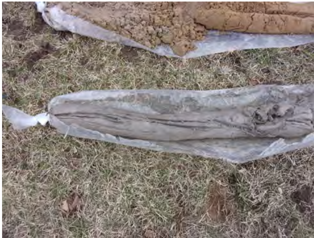
Till clay from 25-30 feet bgs at MW-201 (4/11/2022).
