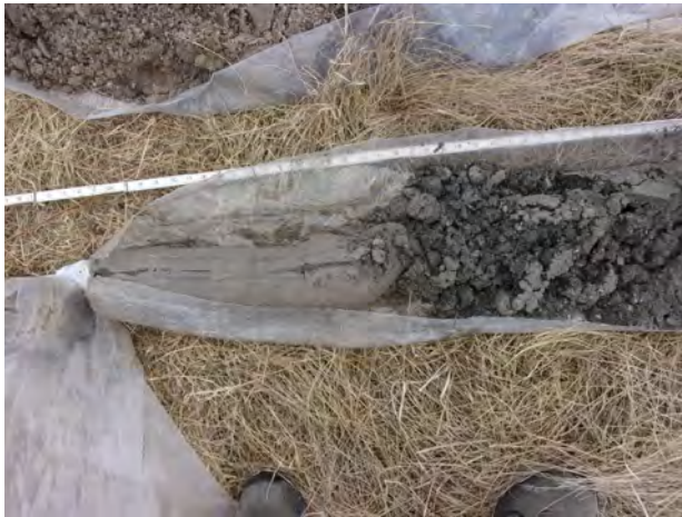
Lacustrine gravelly sand/very hard till clay contact at 33.5 feet bgs at SB-19 (4/12/2022).
