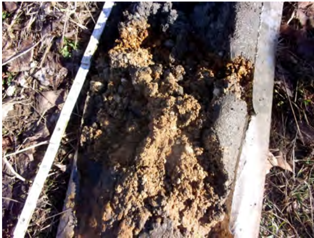
Lacustrine sand from 15.5-20 feet bgs at MW-200 (4/12/2022).
