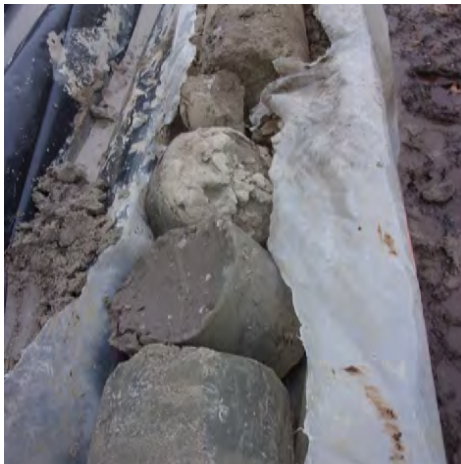
Hardpan-like glacial till from 60-65 feet bgs at MW-300 (4/4/2023).
