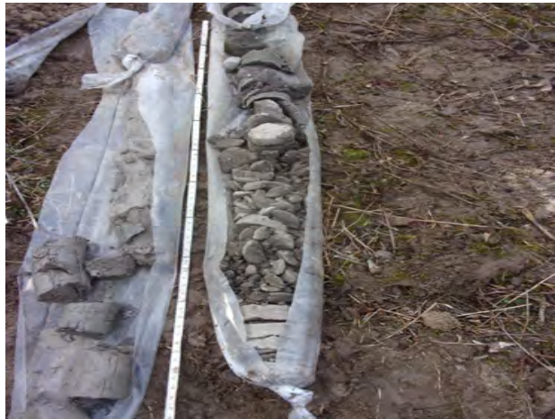
Hardpan-like till clay from 25-30 feet bgs at SB-21 (4/13/2022).
