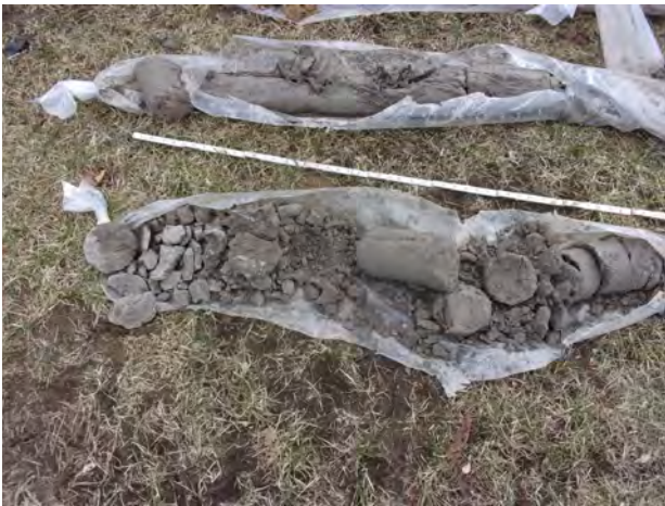
25-30 feet bgs (top) and 35-40 feet bgs (bottom) till clay soil cores from MW-201 (4/11/2022).
