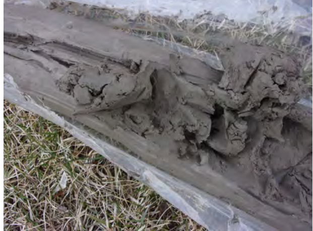
Till clay from 25-30 feet bgs at MW-201 (4/11/2022).
