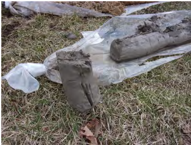
Till clay from 25-30 feet bgs at MW-201 (4/11/2022).
