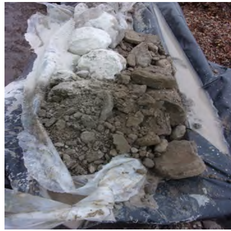
Hardpan-like glacial till and boulder from 80-85 feet bgs at MW-300 (4/4/2023).
