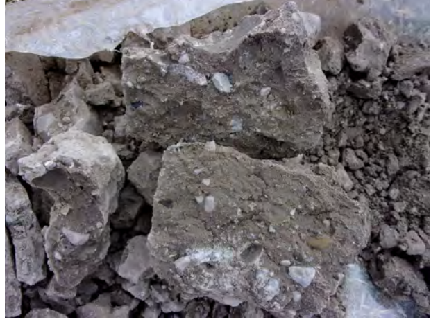
Hardpan-like till clay at 40 feet bgs at MW-201 (4/11/2022).
