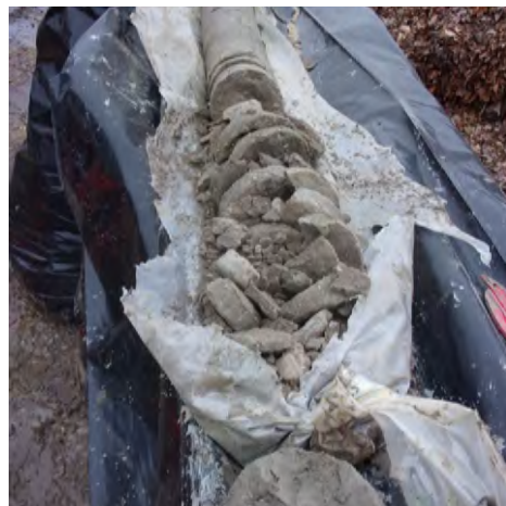
Very hard glacial till clay from 75-80 feet bgs at MW-300 (4/4/2023).
