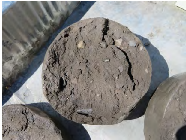
Till clay soil sample from 47-49 feet bgs at SB-19 (4/16/2022).
