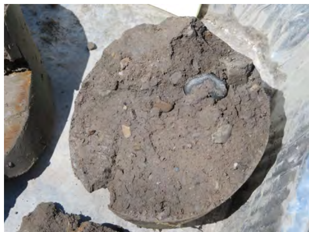
Till clay soil sample from 45-50 feet bgs at SB-20 (4/16/2022).
