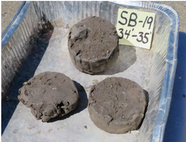
Very hard till soil sample (clayey sand) from 34-35 feet bgs at SB-19 (4/16/2022).
