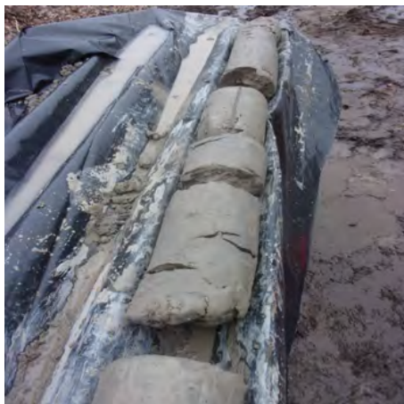
Very hard glacial till clay from 70-75 feet bgs at MW-300 (4/4/2023).
