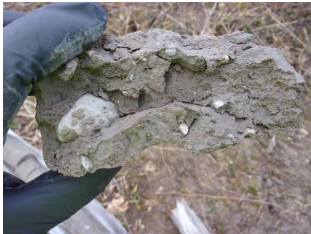
Hardpan-like till clay from 30-35 feet bgs at SB-21 (4/13/2022).
