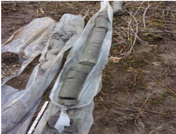
Very hard till clay from 20-25 feet bgs at SB-21 (4/13/2022).
