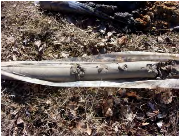
Till clay from 25.5-30 feet bgs at MW-200 (4/12/2022).
