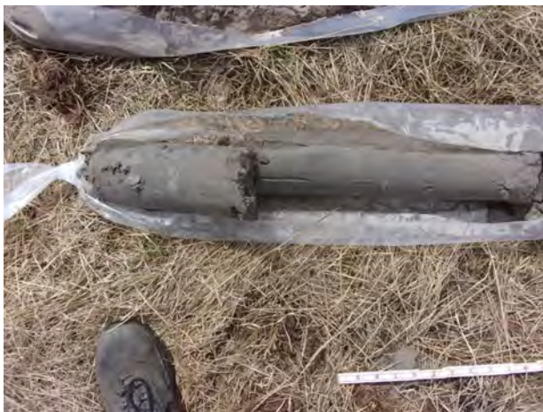
Hardpan-like till clay from 45-50 feet bgs at SB-20 (4/12/2022).
