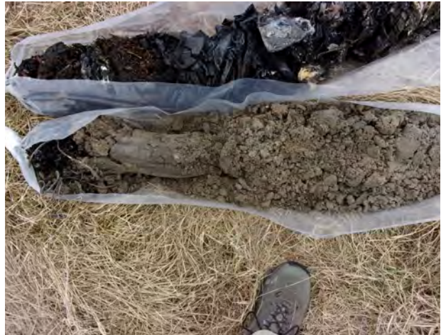
Fill sand and underlying refuse from 17-20 feet bgs at SB-19 (4/12/2022).
