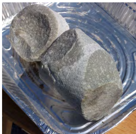
Boulder encountered in MW-300 from approx. from 81-83 ft bgs (4/8/2023).
