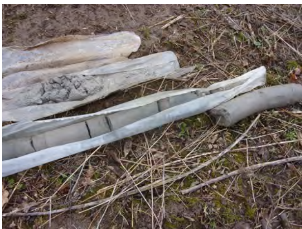
Very hard till clay from 20-25 feet bgs at SB-21 (4/13/2022).
