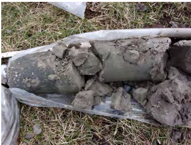
Hardpan-like till clay at 35 feet bgs at MW-201 (4/11/2022).
