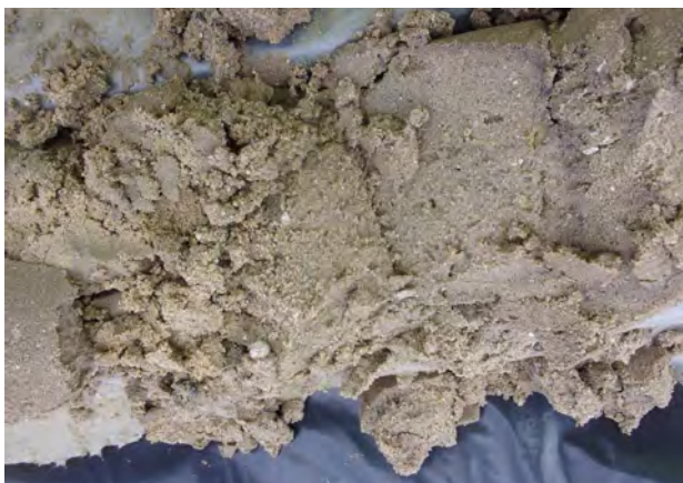
Brown glacial outwash sand from 10.5-14 feet bgs at MW-300 (4/4/2023).
