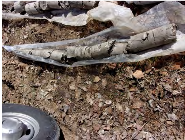
Hardpan-like till clay from 47-50 feet bgs at MW-200 (4/12/2022).
