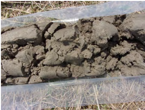
Lacustrine sand at 38 feet bgs at SB-20(4/12/2022).
