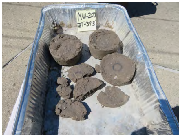
Till clay soil sample from 37-39.5 feet bgs at MW-200 (4/16/2022).
