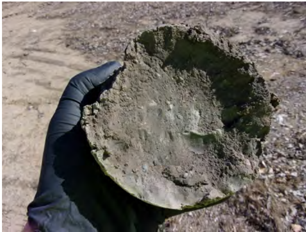
Hardpan-like till clay from 35-39.5 feet bgs at MW-200 (4/12/2022).
