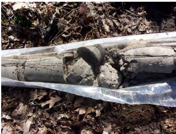
Hardpan-like till clay from 33-35 feet bgs at MW-200 (4/12/2022).
