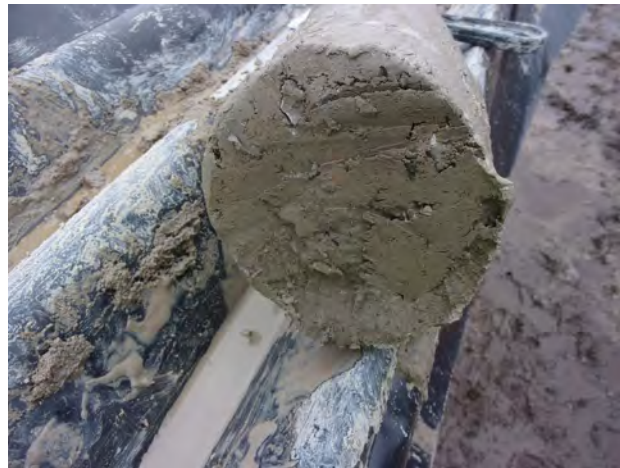
Very hard glacial till clay at 70 feet bgs at MW-300 (4/4/2023).
