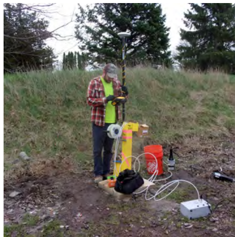
Establishing MW-300 location coordinates with GPS (4/20/2023).
