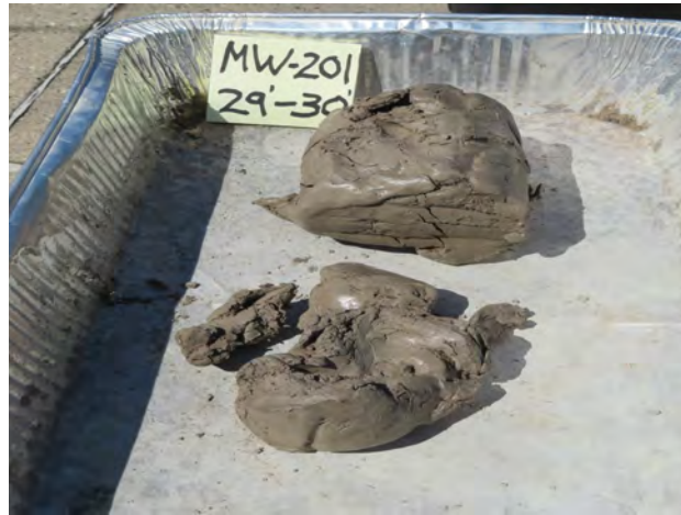
Till clay soil sample from 29-30 feet bgs at MW-201 (4/16/2022).
