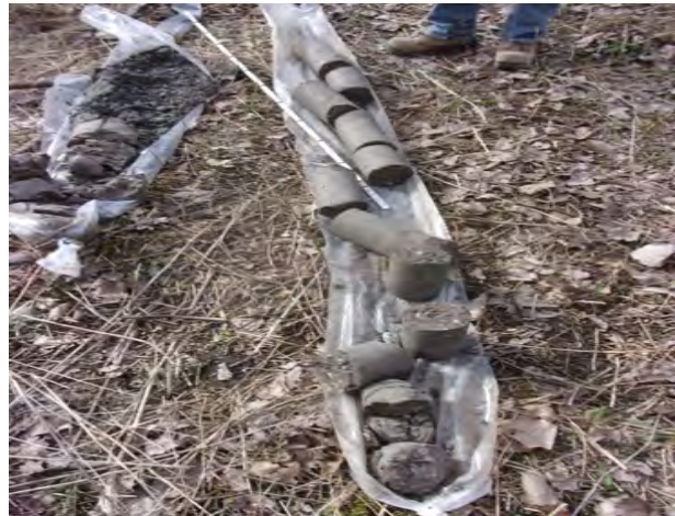
Very hard till clay from 10-15 feet bgs at MW-202 (4/12/2022).
