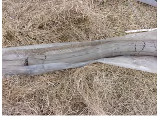
Very hard till clay from 35-40 feet bgs at SB-19 (4/12/2022).
