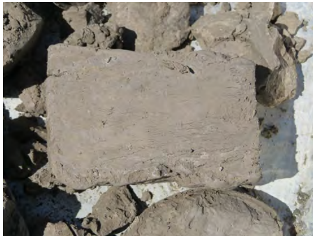
Till clay soil sample from 25.5-30 feet bgs at MW-200 (4/16/2022).
