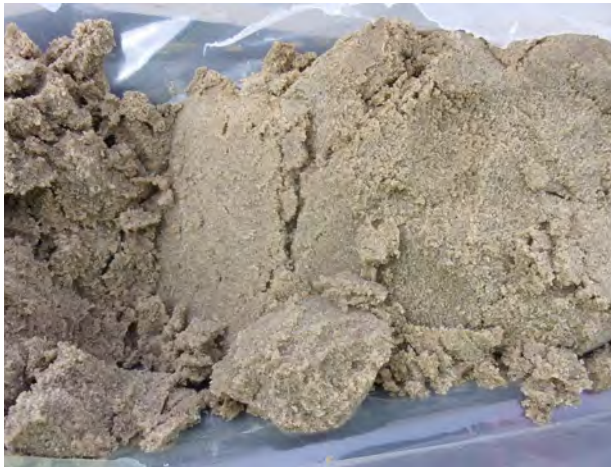
Lt. brown glacial outwash silty fine sand from 14-24.5 feet bgs at MW-300 (4/4/2023).
