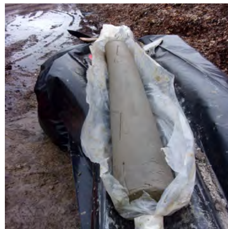
Hard glacial till clay from 45-50 feet bgs at MW-300 (4/4/2023).
