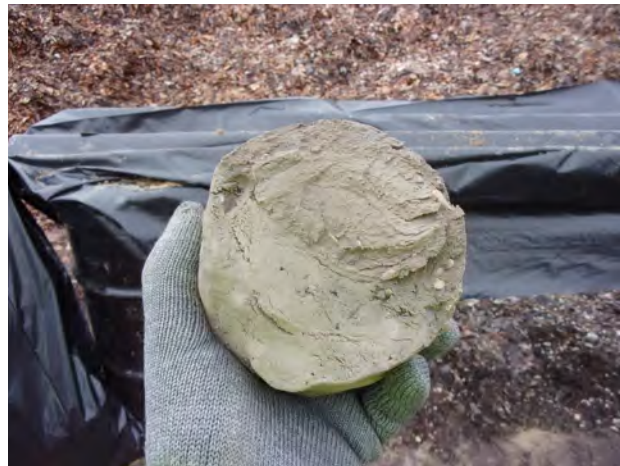
Hard glacial till clay from 25-30 feet bgs at MW-300 (4/4/2023).
