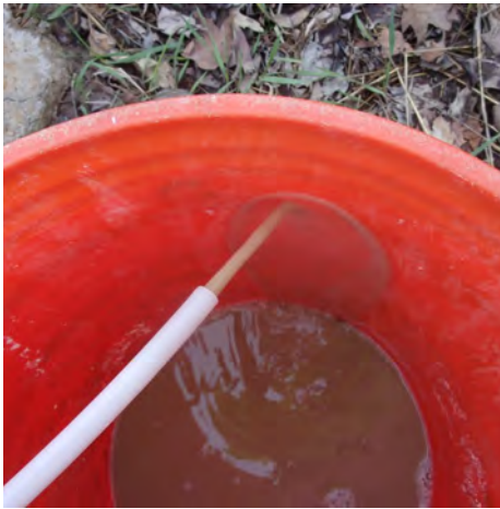
MW-300 Cloudy/Silty Purge Water (4/20/2023).
