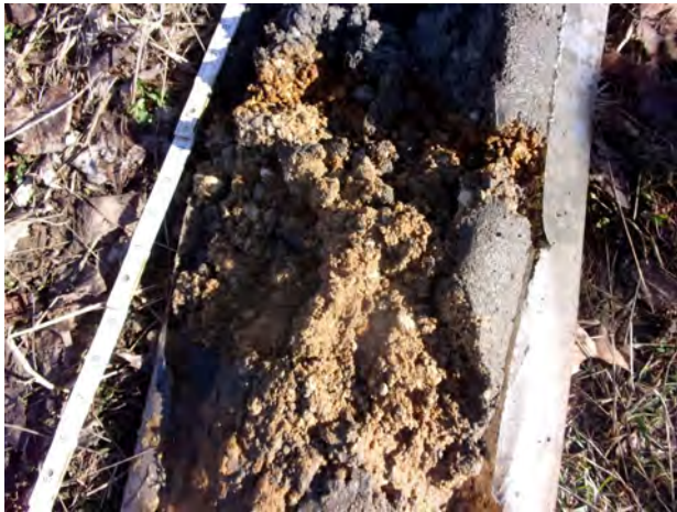
Lacustrine sand from 15.5-20 feet bgs at MW-200 (4/12/2022).
