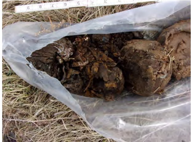
Clay cap (right) and top of refuse (left) from 1.5-2.5 feet bgs at SB-19 (4/12/2022).
