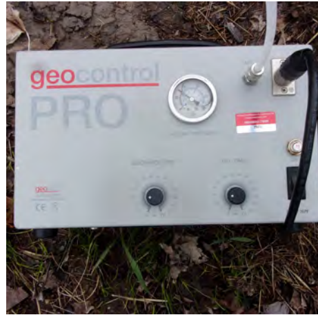
Bladder Pump Controller (4/20/2023).
