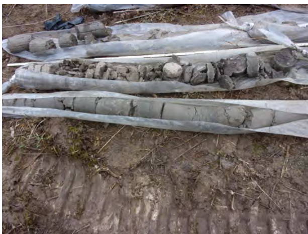
Till clay from 35-40 feet bgs (bottom), 25-30 feet bgs (middle), and 15-20 feet bgs (top) at SB-21 (4/13/2022).
