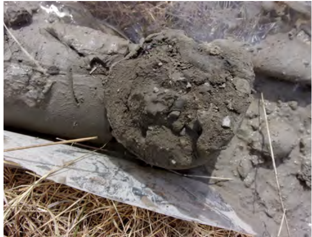
Very hard till clay from 40-44.5 feet bgs at SB-20 (4/12/2022).
