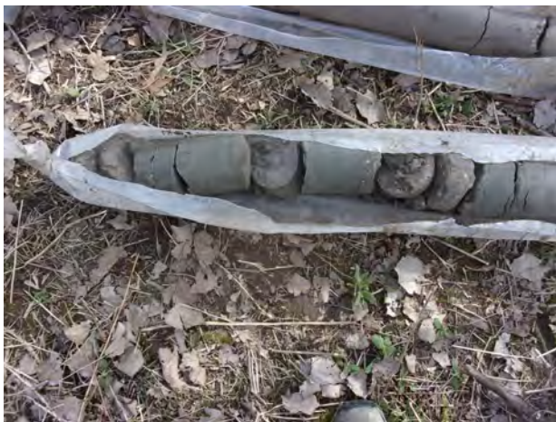
Very hard till clay from 35-40 feet bgs at MW-202 (4/12/2022).
