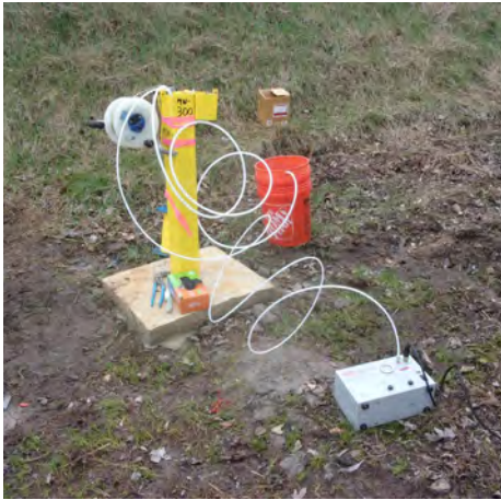
Purging Deep Monitoring Well MW-300 (4/20/2023).
