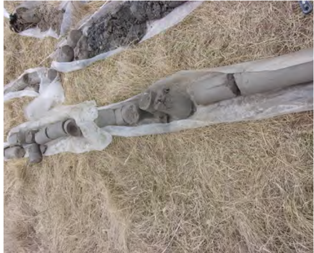
Very hard till clay from 40-50 feet bgs at SB-19 (4/12/2022).
