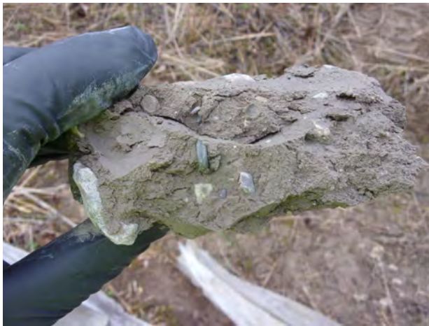
Hardpan-like till clay from 30-35 feet bgs at SB-21 (4/13/2022).
