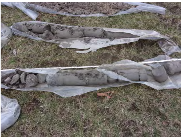
30-35 feet bgs (top) and 40-45 feet bgs (bottom) till clay soil cores from MW-201 (4/11/2022).
