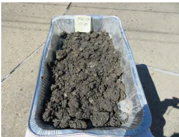
Lacustrine gravelly sand soil sample from 17-20 feet bgs at MW-200 (4/16/2022).
