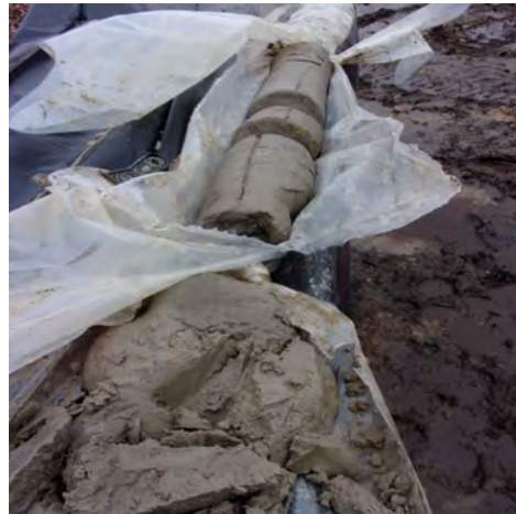
Gray sandy silt (bottom of photo) transitioning to gray glacial till clay at 25 feet bgs at MW-300 (4/4/2023).
