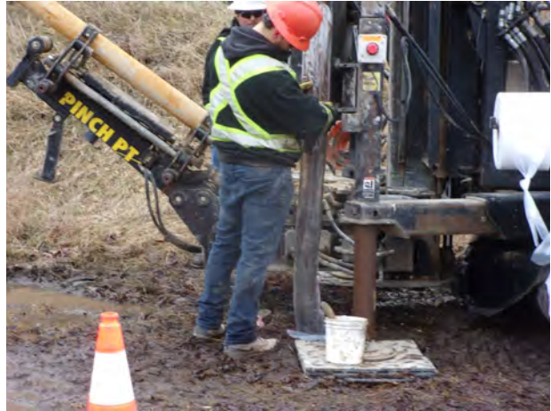
Retrieving soil core sample (4/4/2023).
