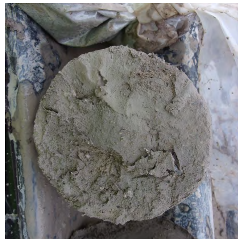
Very hard glacial till clay at 80 feet bgs at MW-300 (4/4/2023).
