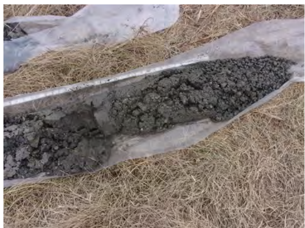
Lacustrine gravelly sand from 30-32 feet bgs at SB-19 (4/12/2022).
