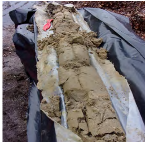
Brown glacial outwash sand from 10.5-14 feet bgs at MW-300 (4/4/2023).
