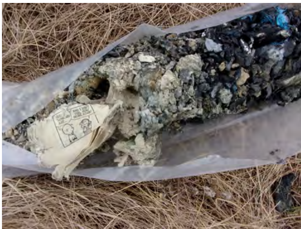
Refuse from 10-15 feet bgs at SB-19 (4/12/2022).
