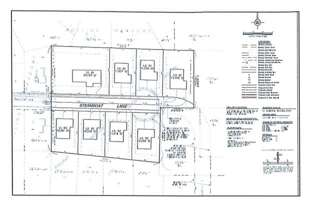
Mr. Grittman stated the plan shows a temporary cul-de-sac along the proposed new street that serves Lot 3, Block 1 on the north, Lot 4, Block 1 at the end of the cul-de-sac with an extended driveway through the residual right of way, and also Lot 4, Block 2 on the south side of the street. Notes on the plat state that the cul-de-sac would be removed at the time of extension of the street, which will be a condition of preliminary plat approval.
