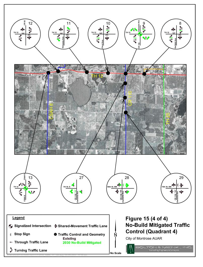
operations and there would need to be channelized right turns on the south and east legs of the intersection. A double-lane roundabout would also be an option.
