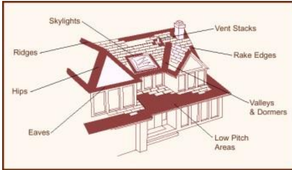
FIGURE 2-2 Underlayment for Asphalt Shingles.
