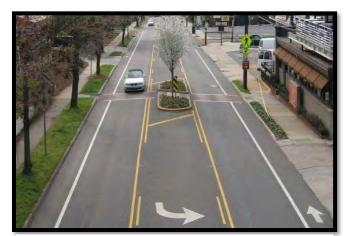
Figure 23. Median island providing pedestrian refuge on a three-lane section with center turn-lane. *Source:*
