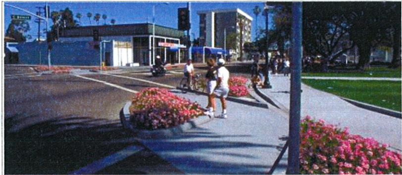
**Narrowing Travel Lanes.** Conventional traffic engineering has recommended travel lanes that are 12' wide (or greater) to meet safety standards, but newer evidence shows that lanes as narrow as 9' can still be safe for driving. Narrowing lanes also allows space for addition of bicycle lanes and improves crossing for pedestrians and gives them more space to walk.
