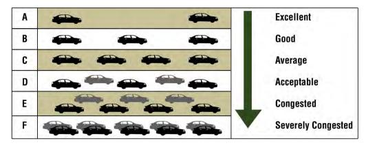
Roadway segment LOS and intersection LOS differ in the way they are measured. Roadway segment LOS relates directly to the number of lanes in the segment and is determined by a volume/capacity ratio. Where the number of vehicles traveling on a roadway exceeds the number of vehicles that can be reasonably accommodated without undue speed reduction, the roadway is defined as LOS F.
