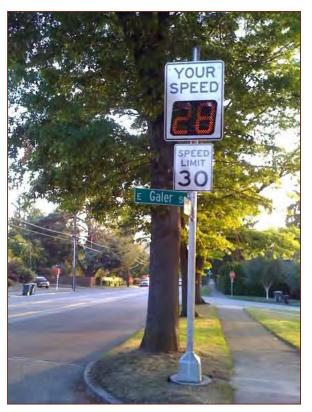
The RADAR SPEED SIGN is very similar in nature to the radar trailer device. The notable difference between this device and the radar speed trailer is that the radar speed sign in not portable. The device can also have the ability to store data over time to provide speed data to the City. This device measures and records a vehicles speed and displays it next to the posted speed limit sign reminding vehicles to slow to the appropriate speed
