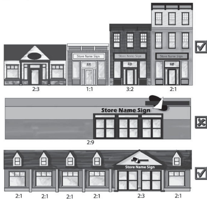
Figure 13: These three elevations illustrate proper and improper articulation and proportions for buildings in the District
