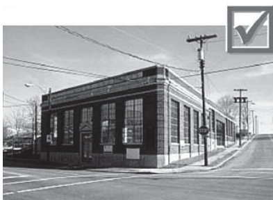
Figure 14: This building shows how a tall, single story building can be well articulated through the use of tall windows. This approach is preferred over the use of a faux upper story
