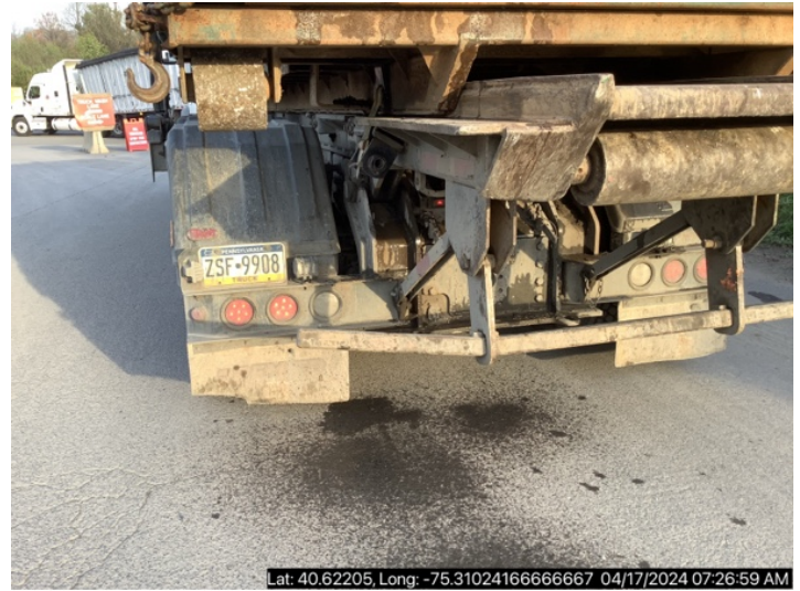
#: Photo # 4: leak from rear tailgate.
