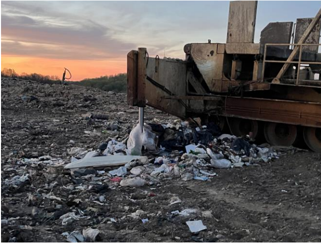
Photo 5: Exposed waste around the base of the tipper.
