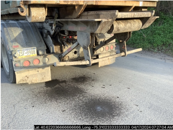
#: Photo # 3: leak from rear tailgate.
