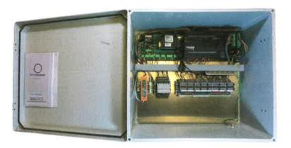
The HTT-4100 is typically used for treatment plant monitoring. The base model comes with equipped with 28 discrete inputs, 12 analog inputs, and 8 discrete outputs. Optional modules can be added to increase all three signal types. The HTT-4100 also has an optional local touch screen for data monitoring and controls. The HTT-4100 works seamlessly with the High Tide Technologies TelemetyVIEW web interface.
