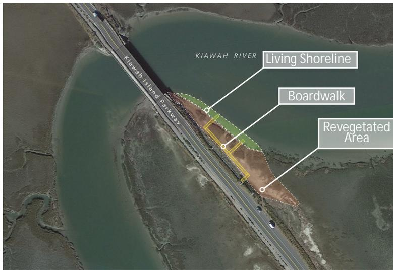
**Left:** The causeway entrance to Kiawah Island is experiencing significant degradation due to erosion caused by trampling. Over time, and coupled with SLR, the parkway infrastructure could be compromised by a sharp decline in marsh health, accelerating erosion. Management techniques could include the thoughtful design of public access (e.g. boardwalk or fenced path), paired with the use of previously detailed restoration techniques, such as revegetation and living shoreline.
