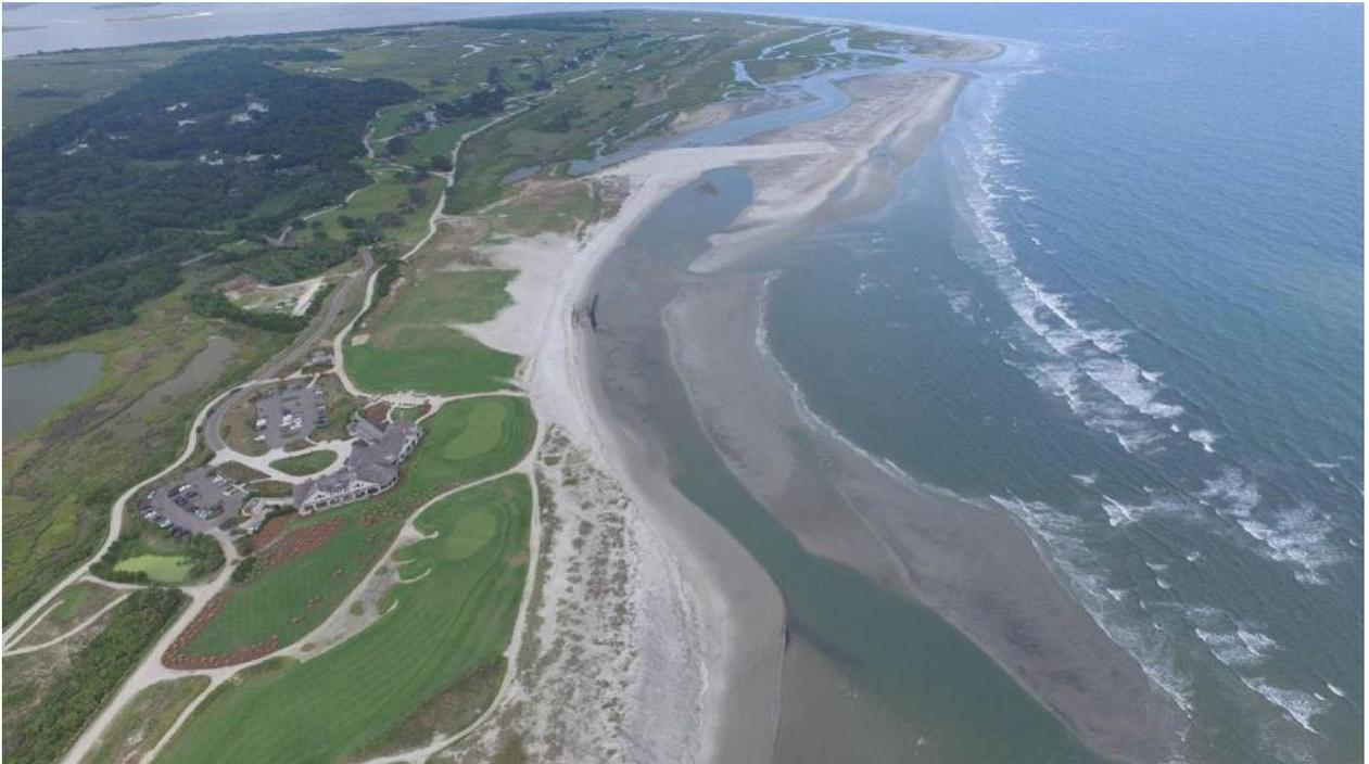
Aerial image of the completed 2015 channel relocation project in July 2015. The new inlet was opened ~3,000 ft east of the old channel.
