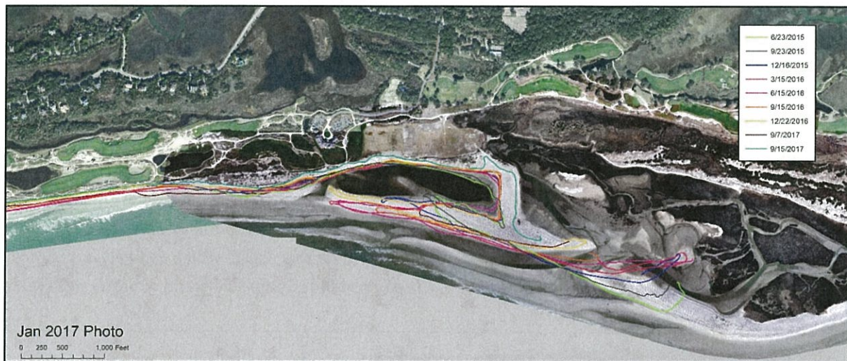
FIGURE 4.3. Position of the dune line or line of stable dry beach from June 2015 to September 2017. Data were collected by Town staff. The inlet has migrated over 1,400 ft to the west.
