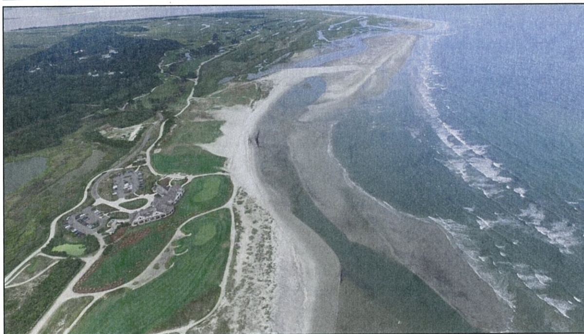
FIGURE 2.10. Aerial image of the completed 2015 channel relocation project in July 2015. The new inlet was opened ~3,000 ft east of the old channel.
