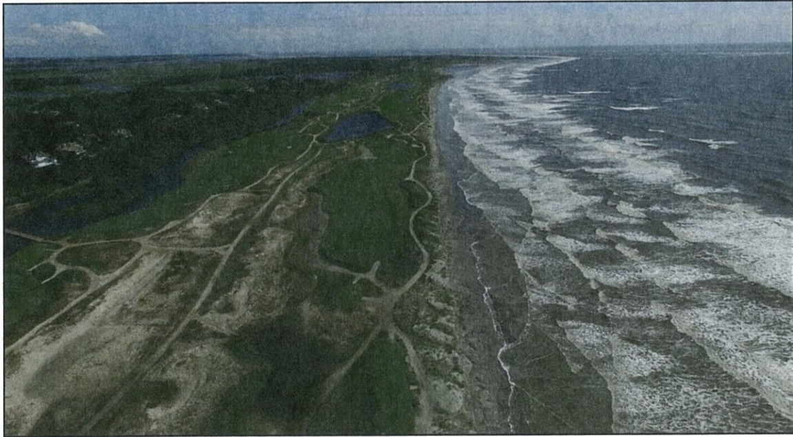
FIGURE 4.15. September 2017 aerial image of the Ocean Course Reach following Hurricane Irma . The storm eroded dunes along the course and, in one location, reached the cart path.
