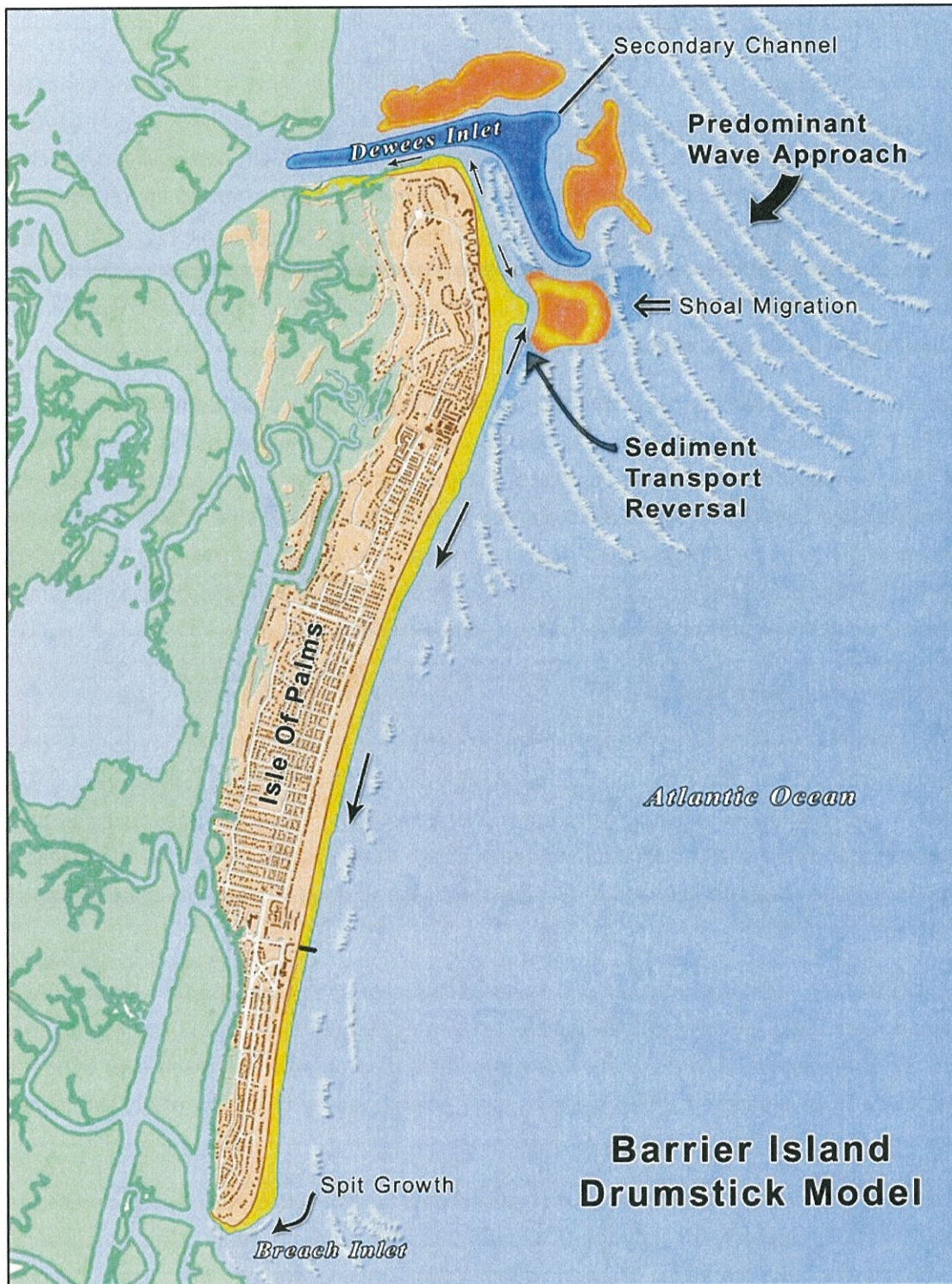
FIGURE 2.2. Barrier-island drumstick model (after Hayes 1977) using Isle of Palms as an example. The upcoast end is wider due to additions of sand from shoal-bypass events in the inlet. Net transport to the south builds a spit at the downcoast end of the island.
