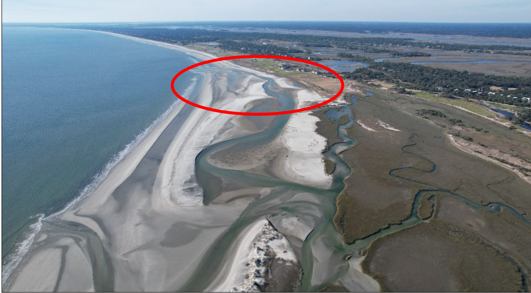
FIGURE 4.9. The Ocean Course Reach lies along the transition zone from the ‘strand’ beach to the east end of the driving range. In January 2019, the lagoon and flushing channel fronting the Ocean Course Club House was nearly cut off from the ocean. However, between January 2019 and November 2020, a new flushing channel opened naturally (red circle) and presently is draining the lagoon. (photo via UAV December 2024)
