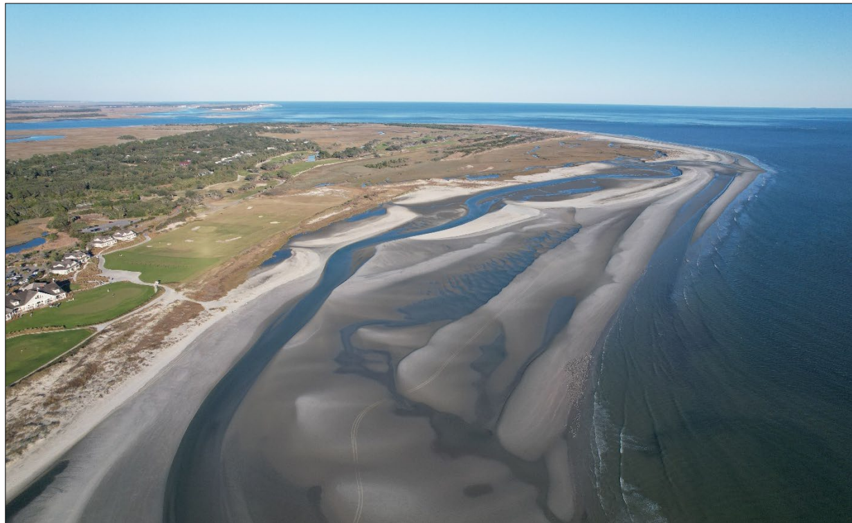
FIGURE 4.12. October 2017 aerial image [UPPER] compared to December 2024 aerial image [LOWER] of the Ocean Course Reach (eastern half). The ponded area is the relict channel basin from the 2015 project, formed before the closure dike was constructed. By December 2024, a similar flushing channel has formed close to the 2015 channel location, which triggered remedial work to close it. The present channel may have to be redirected similarly in the next 2–3 years.
