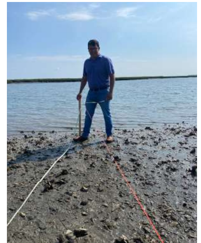
Weston & Sampson staff measure slope on site using a line level.
