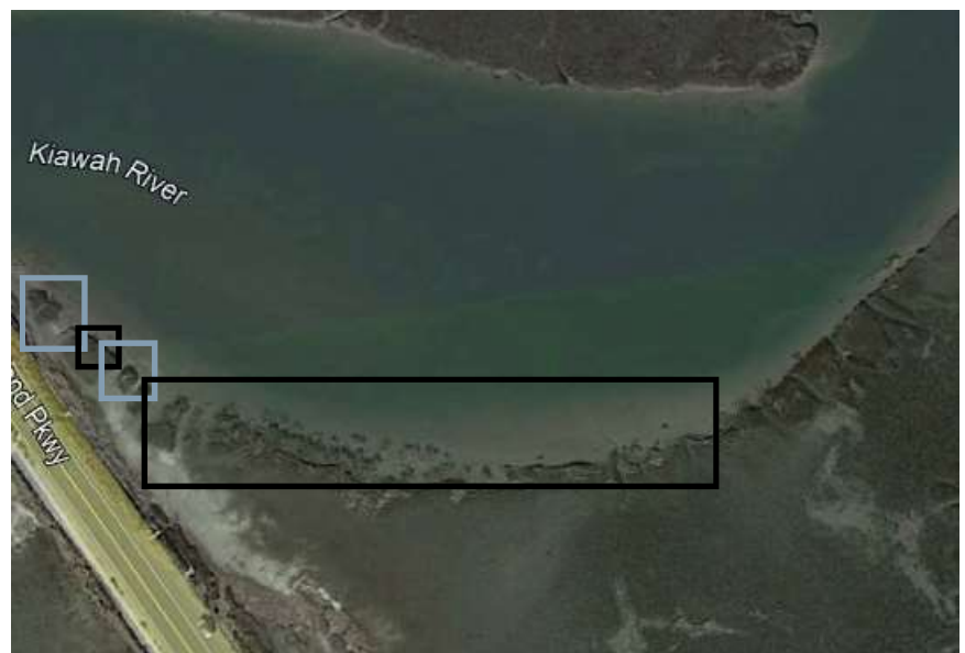
This photo is of very soft/moderately soft substrate. Sinkability is high. Any living shoreline materials applied in this area should be light in weight.
