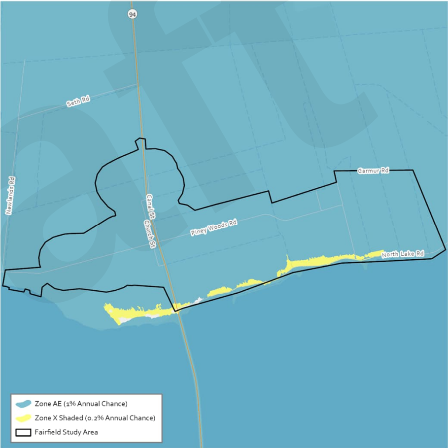
Fairfield - 97% land area in the Special Flood Hazard Area
