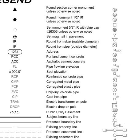
Water main manhole Monitoring well Yard hydrant Gas meter Gas valve Air conditioning unit Electric manhole Electric meter Electric pedestal Electric transformer Utility hand hole Utility pole Light pole Utility pole with light Light pole with double arm Light pole with single arm Ground light Traffic signal Traffic signal with light Traffic manhole Communication pedesta Street sign Basketball hoop
