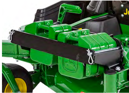
Standard weight bracket and weights, for dump-from-seat MCS
