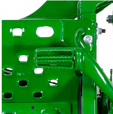
Mower lift pedal
