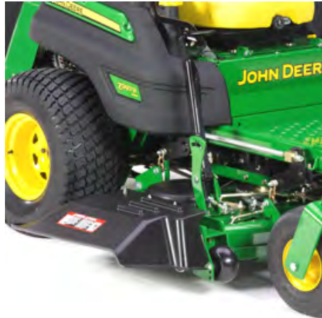
Mulch On Demand control lever (shown on Z997R)
