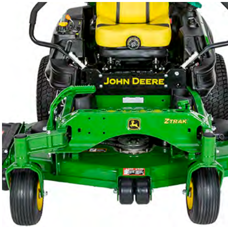
Front axle and caster wheels
