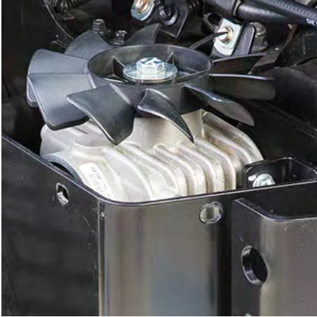
Cooling fins and fan for right-angle gearbox
