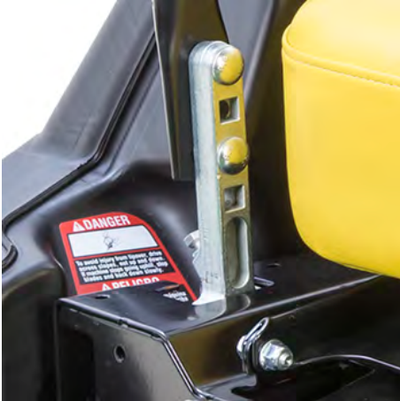
Motion-control lever two-position height adjustment
