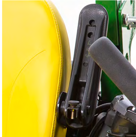
Armrest raised to show adjustment feature
