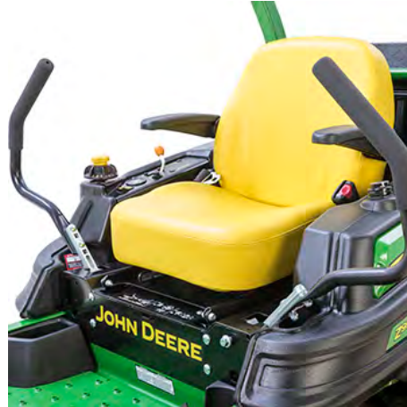
Motion-control levers in park position
