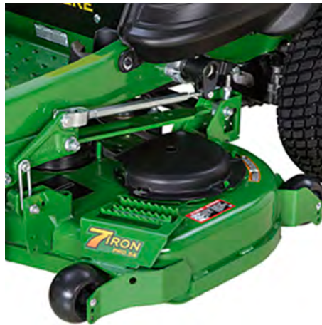
Reinforcement welded on left end of mower
