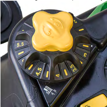
Mower deck height adjustment knob
