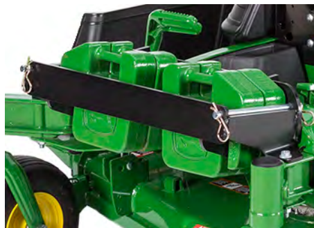
Standard weight bracket and weights, for three-bag MCS
