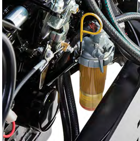
Engine oil filter, dipstick, and fuel filter/water separator
