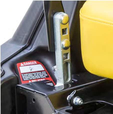
Motion-control lever height adjustment bolts
