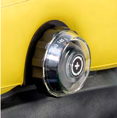
Mechanical suspension seat adjustment
