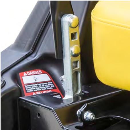
Motion-control lever height and fore/aft adjustment bolts
