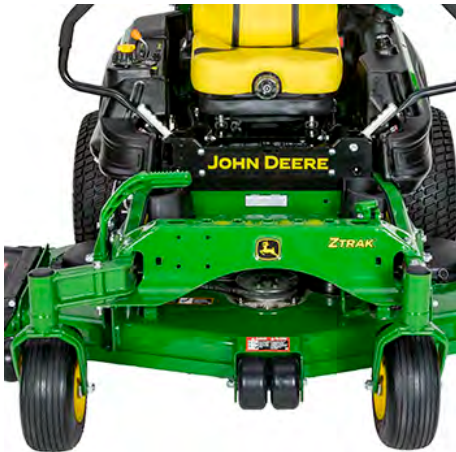
Front axle and caster wheels
