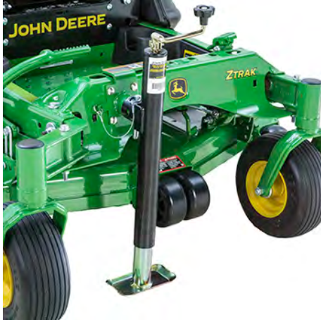
Jack kit and jack installed
