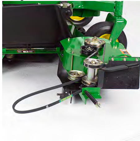
Power Flow blower in cleanout position
