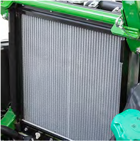
Radiator shown with debris screen removed
