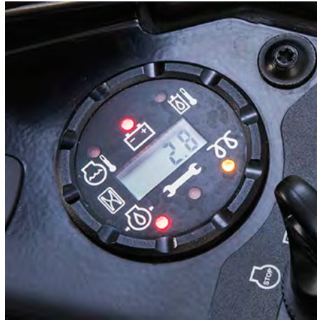
Hour meter, monitoring, and diagnostic display
