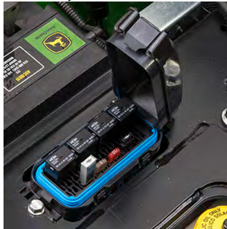
Sealed fuse and relay box
