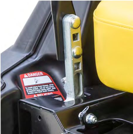
Motion-control lever height adjustment bolts
