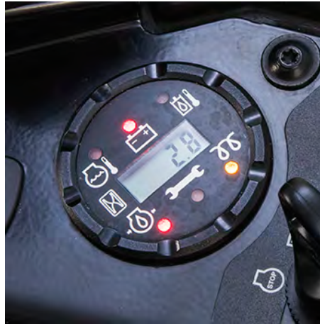
Hour meter, monitoring, and diagnostic display
