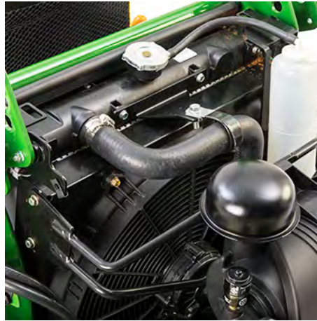
Radiator and electric cooling fan
