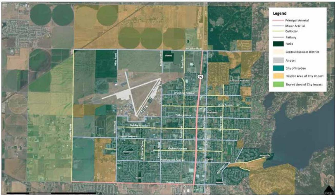
**Figure 7-1: Functional Classification Roadway System**
