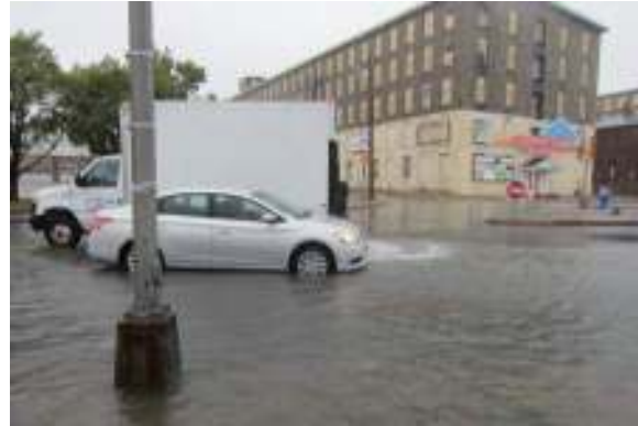
Chronic ponding/flooding in Stafford Square occurs due to the “bowl” shape of drainage basin and insufficient sewer and drain capacities.
