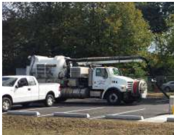
Vector trucks are used for pipe and catch basin cleaning, and other maintenance activities.
