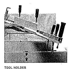
Convenient, drop-in tool holder is located on the rear of the machine and keeps all tools necessary for routine maintenance (including blade changes) within reach.
