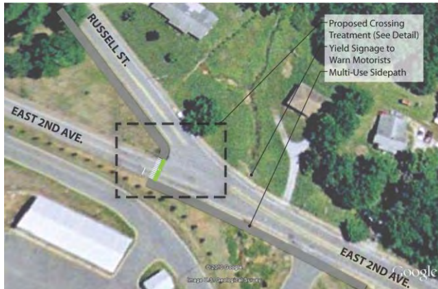
The conceptual crossing at East 2nd Avenue employs signage, striping, and a painted “crossbike” to guide users across the intersection.
