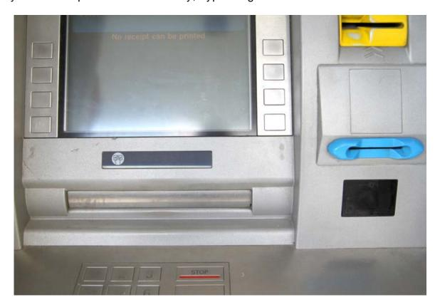
The above picture is a real-life skimmer in use on an ATM. You can see how the arrows are very close to the reader. That is a sign a skimmer was installed over the existing one, since the real card reader would have some space before the arrows.
