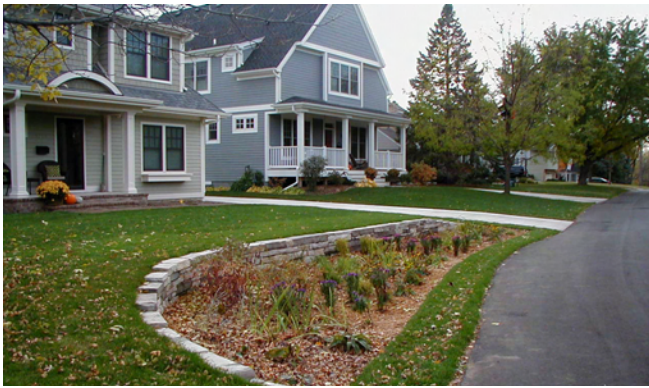
Grass filter strip between road and rain garden
