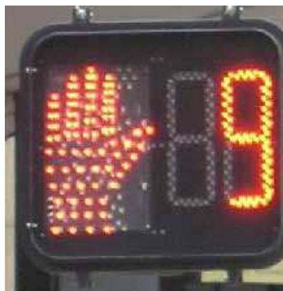
Countdown pedestrian signals convey the actual time a pedestrian has to safely make it through the intersection.
